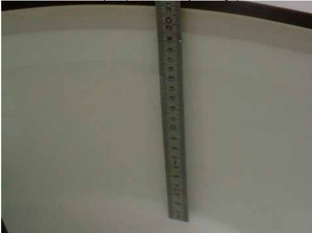
Photo 4: Liquid depth 2450 MHz body simulating liquid
