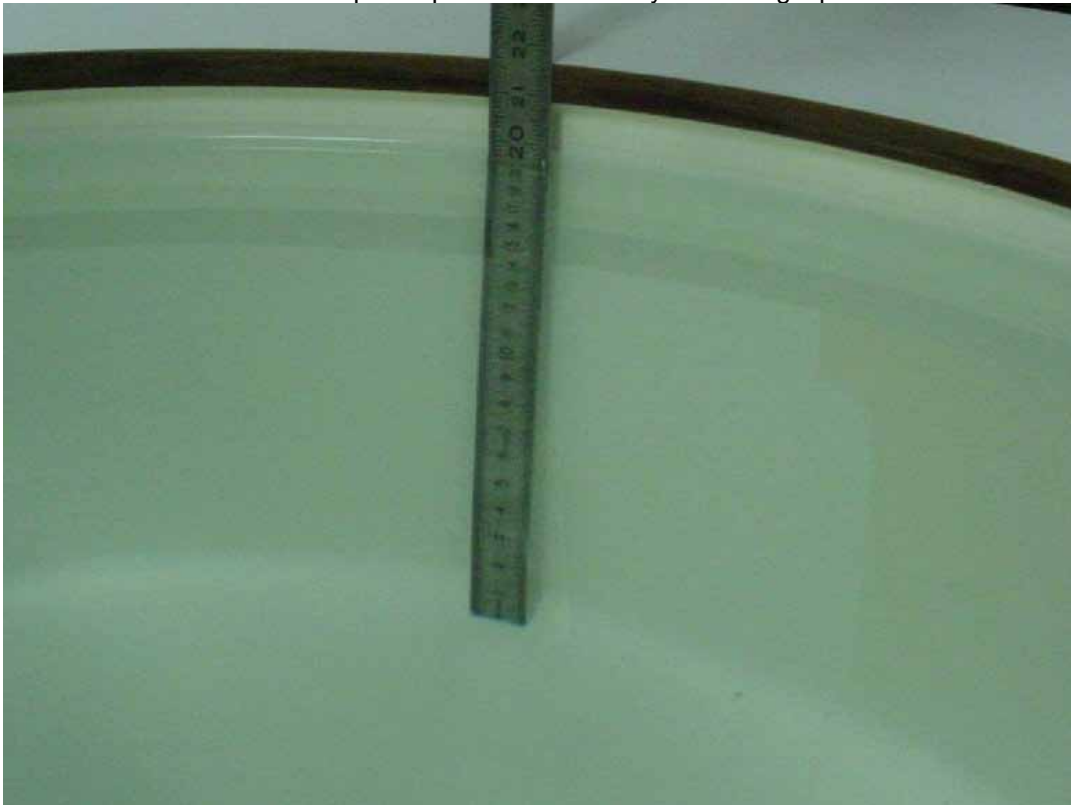
Photo 4: Liquid depth 2450 MHz body simulating liquid
