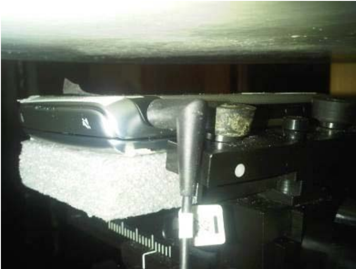
Figure E12. Body-worn configuration (No Holster, Headset #3, 15mm away, back facing phantom)
