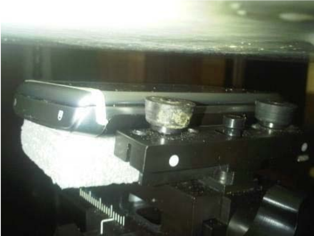
Figure E13. Body-worn configuration (No Holster, 15mm away, front facing phantom)
