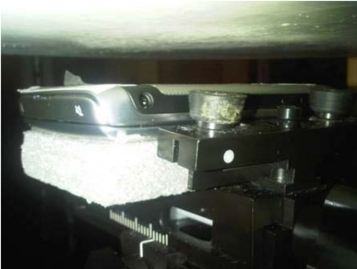
Figure E8. Body-worn configuration (No Holster, 15mm away, back facing phantom)
