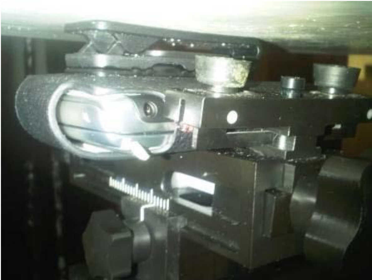
Figure E9. Body-worn configuration (Vertical Holster, back facing phantom)
