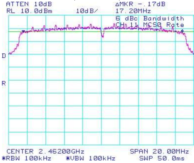
Figure 4-9: 6 dB Bandwidth 802.11n, Channel 11, MCS 0
