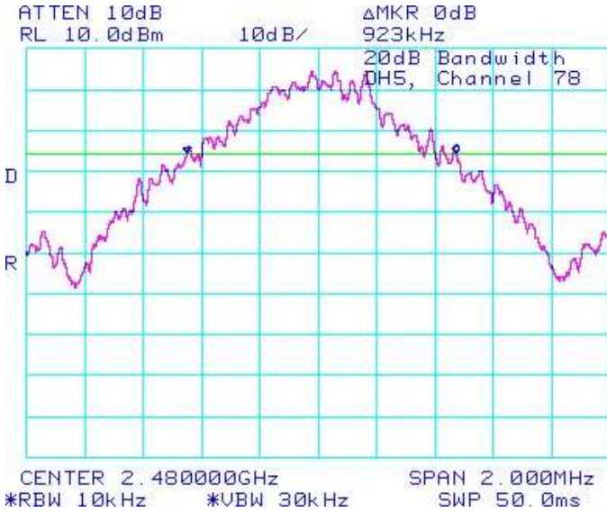
Figure 3-3: 20 dB Bandwidth Single freq., Static PBRs, DH5
