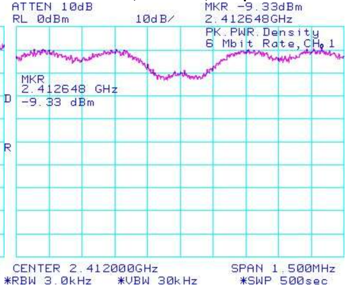
Figure 4-17: Peak Power Spectral Density 802.11b, Channel 6, 1 Mbps
