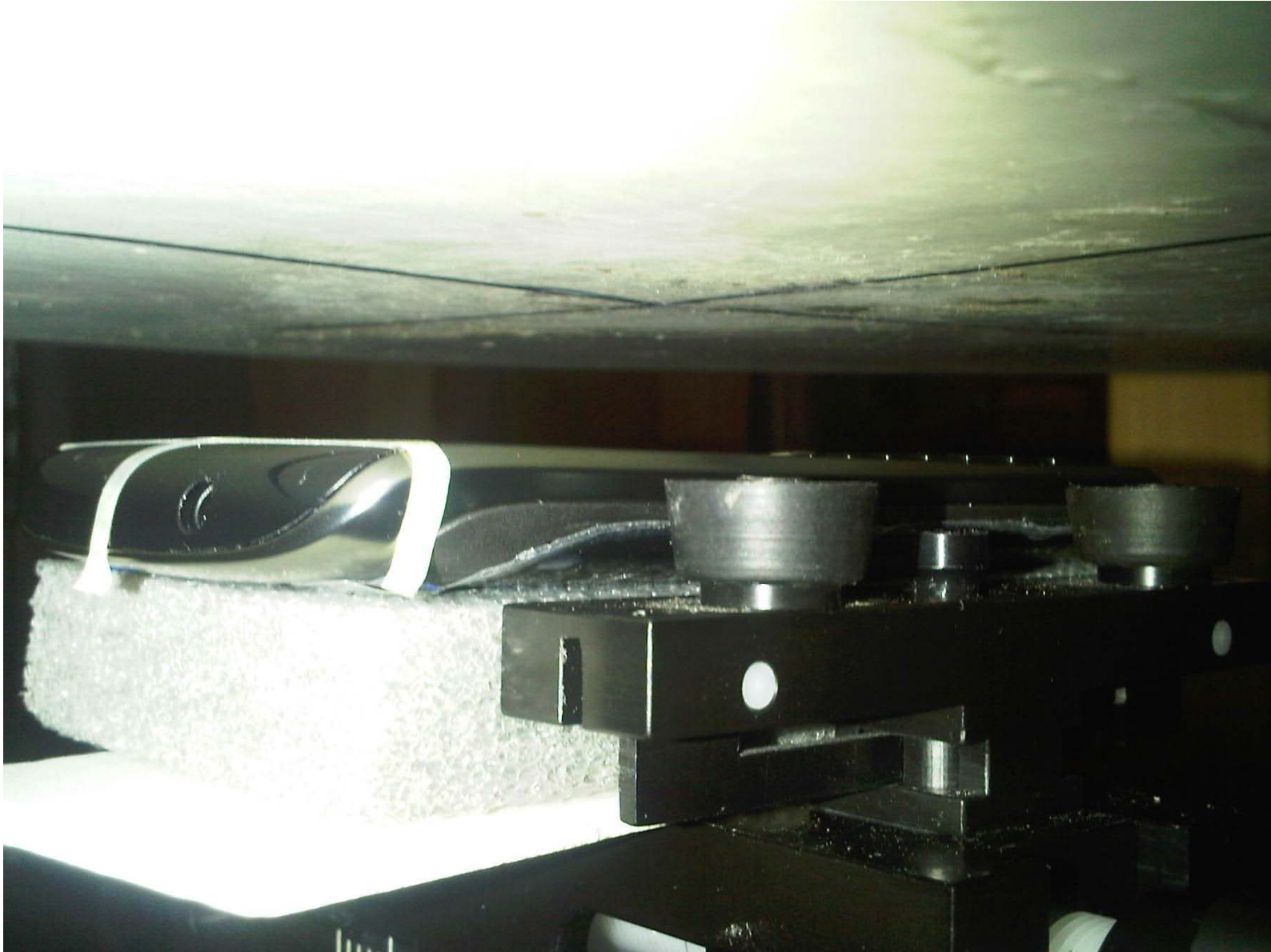
Figure E8. Body-worn configuration (No Holster, front side 15mm away)
