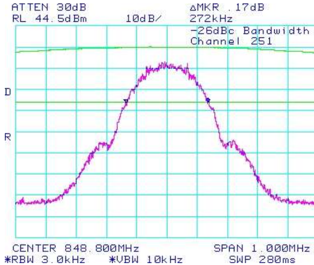
Figure 1-17a: -26dBc bandwidth, GSM850 band High Channel in GSM mode
