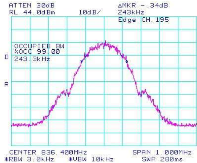
Figure 1-30a: Occupied Bandwidth, GSM850 Band, Middle Channel in EDGE mode
