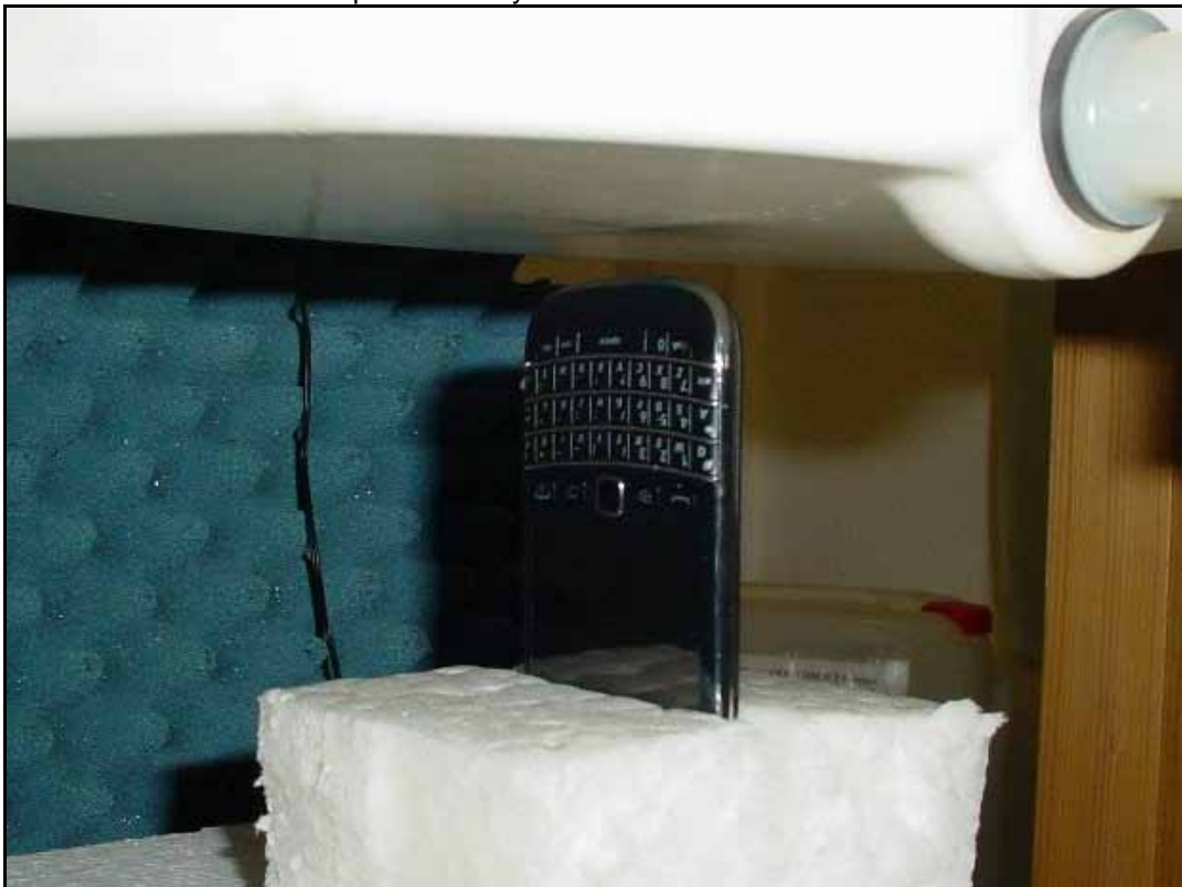
Photo 12: Test position body worn bottom side with 10 mm distance
