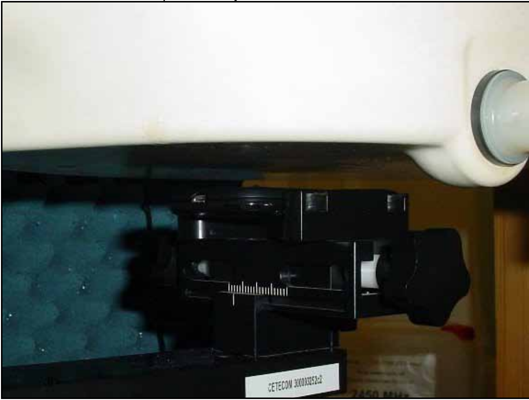
Photo 10: Test position body worn left side with 10 mm distance
