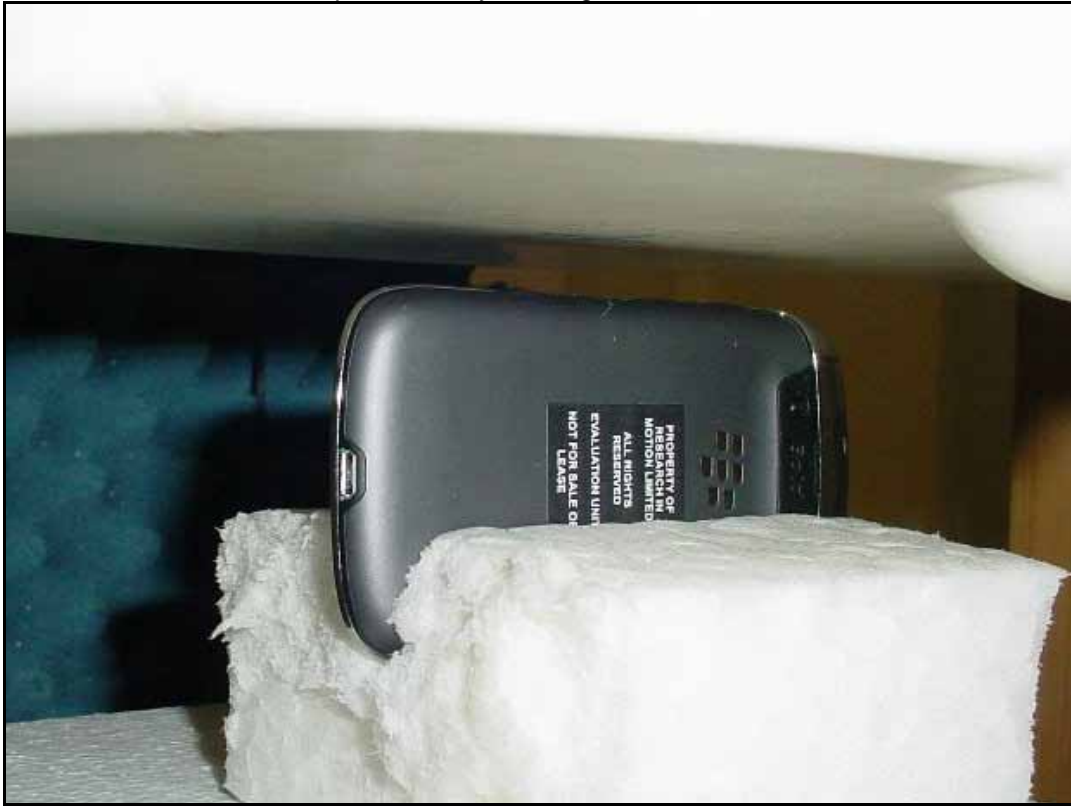
Photo 12: Test position body worn bottom side with 10 mm distance
