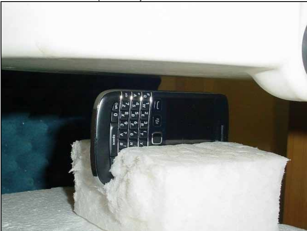
Photo 10: Test position body worn left side with 10 mm distance
