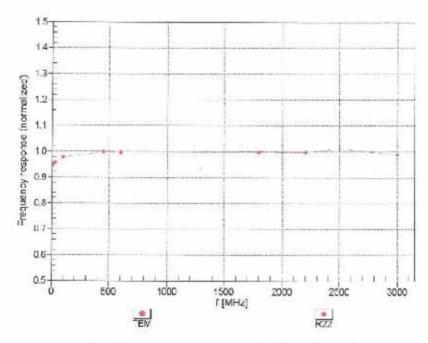
Uncortainty of Frequency Response of E-field: \* 6.3% (k=2)
