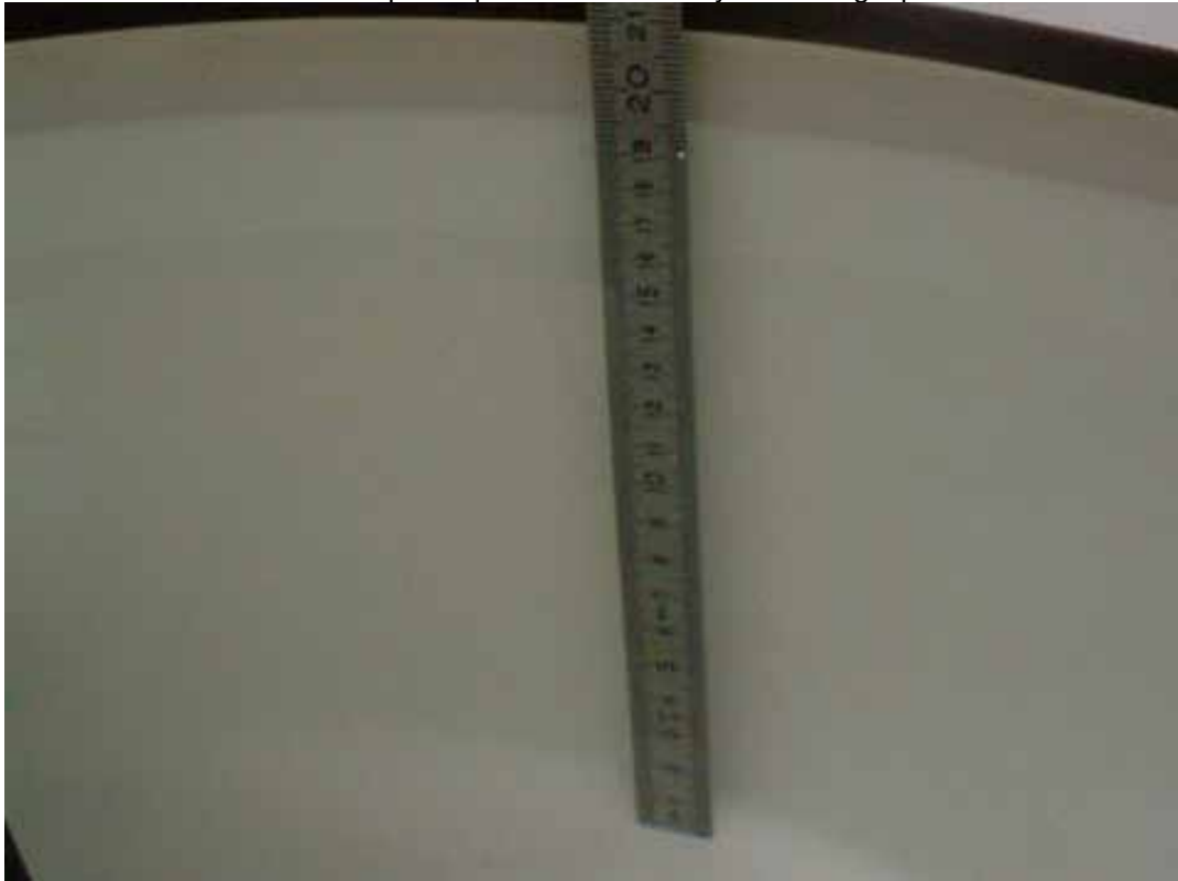
Photo 4: Liquid depth 2450 MHz body simulating liquid
