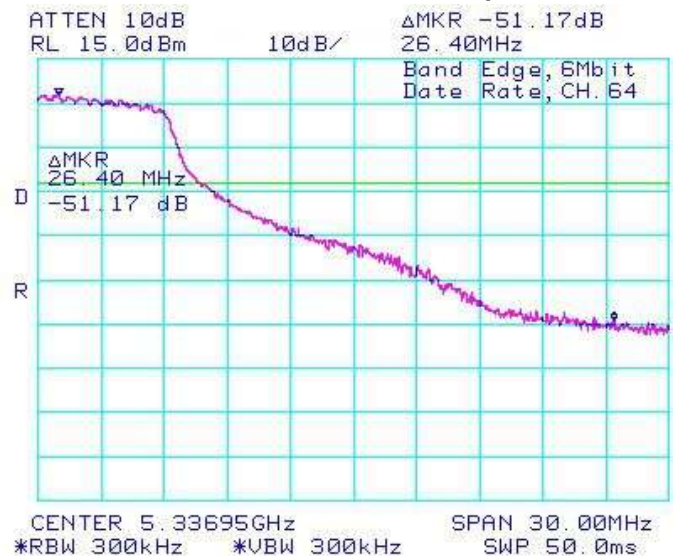
Figure 6-15: Band Edge Compliance
