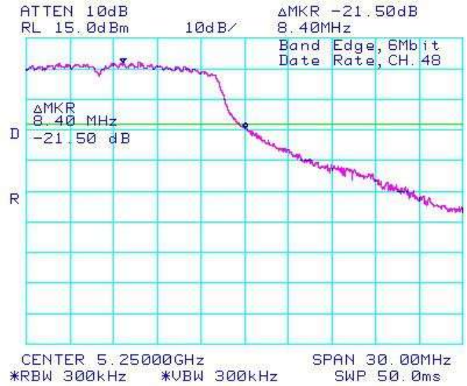
Figure 6-13: Band Edge Compliance
