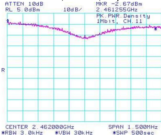
Figure 5-18: Peak Power Spectral Density 802.11b, Channel 11, 1 Mbps
