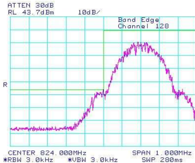
Figure 1-25a: GSM850 band, Low Channel Mask in GSM mode
