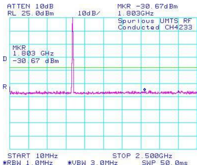
Figure 1-5c: Band 5, Spurious Conducted Emissions, High Channel
