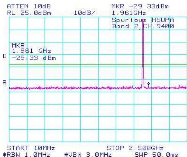
Figure 1-31b: Band 2, Spurious Conducted Emissions, Middle Channel
