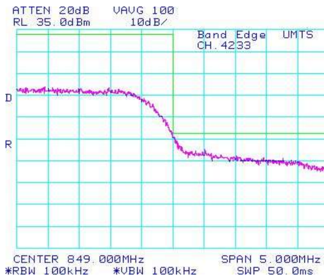
Figure 1-28c: Band 5 High Channel Mask
