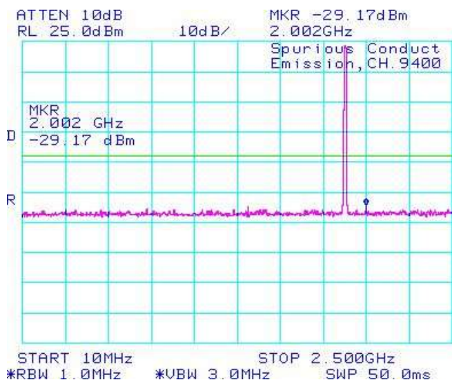
Figure 1-9c: BAND 2, Spurious Conducted Emissions, Middle Channel
