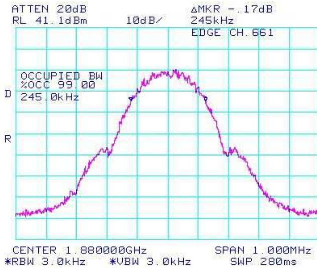
Figure 1-33a: Occupied Bandwidth, PCS1900 Band, Middle Channel in EDGE mode
