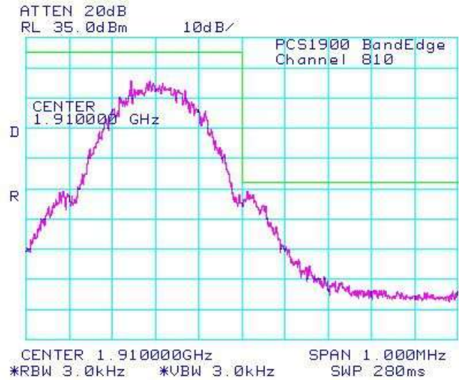
Figure 1-38a: PCS1900 Band, High Channel Mask in EDGE mode
