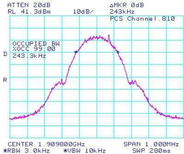
Figure 1-24a: Occupied Bandwidth, PCS1900 High Channel in GSM mode
