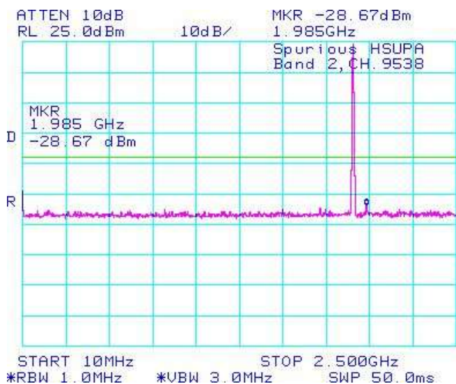
Figure 1-33b: Band 2, Spurious Conducted Emissions, High Channel
