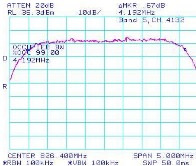
Figure 1-13c: Occupied Bandwidth, Band 5 Low Channel
