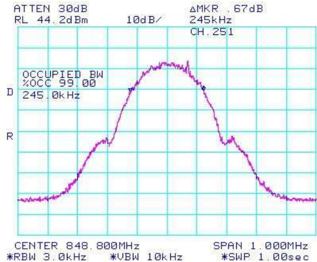
Figure 1-18a: Occupied Bandwidth, GSM850 band High Channel in GSM mode
