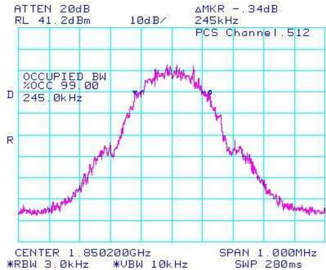
Figure 1-20a: Occupied Bandwidth, PCS1900 Low Channel in GSM mode
