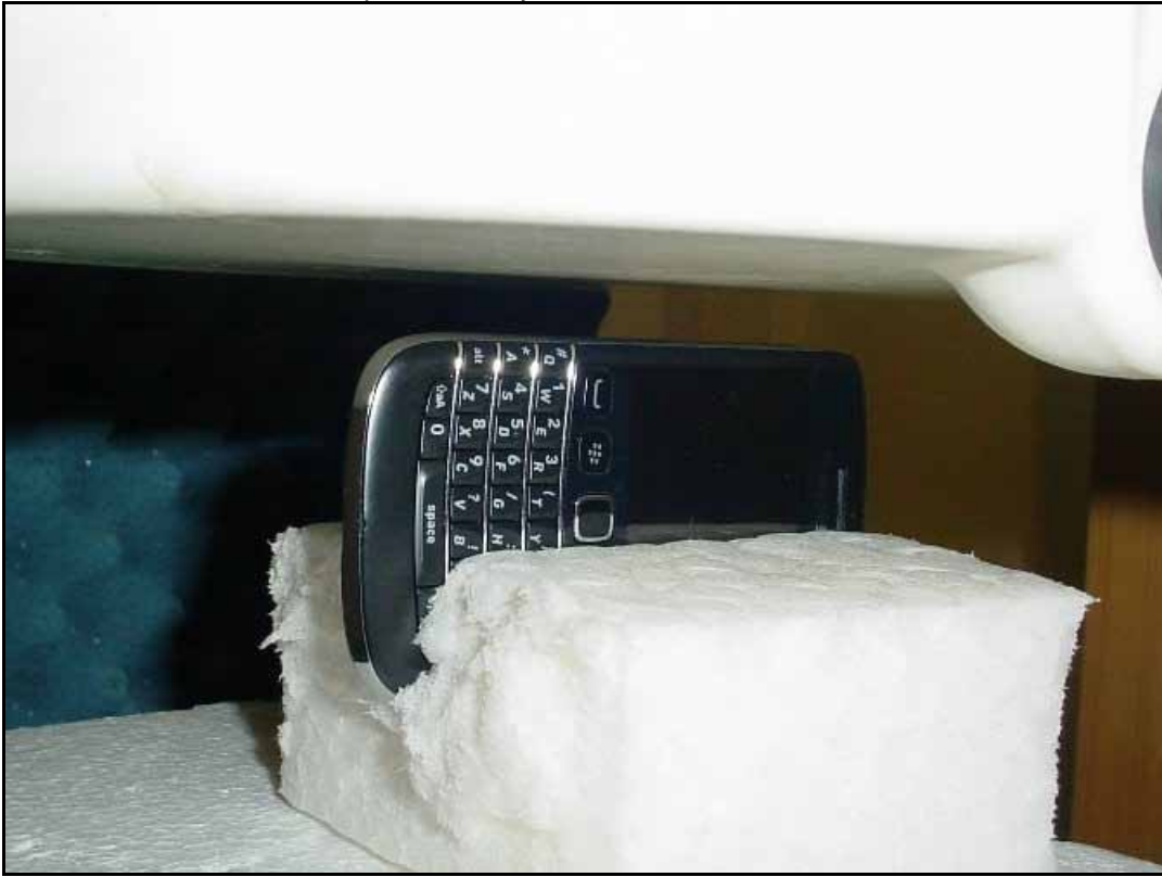
Photo 10: Test position body worn right side with 10 mm distance
