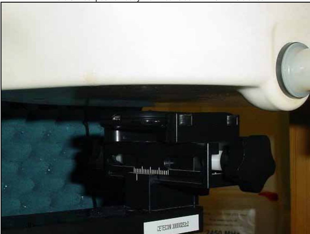
Photo 8: Test position body worn rear side with 10 mm distance
