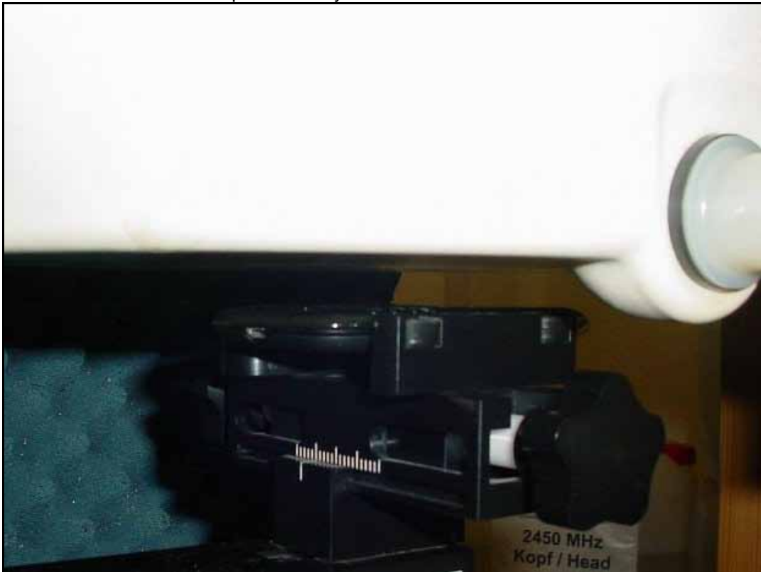
Photo 8: Test position body worn rear side with 10 mm distance
