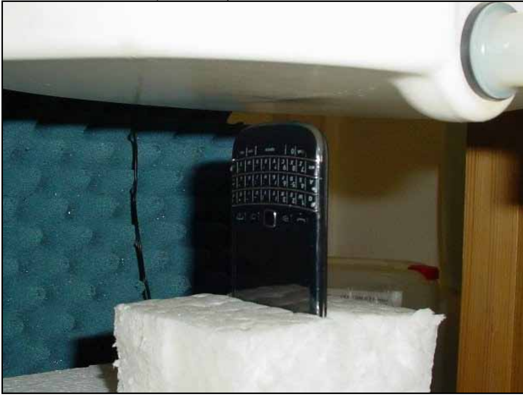
Photo 11: Test position body worn bottom side with 10 mm distance
