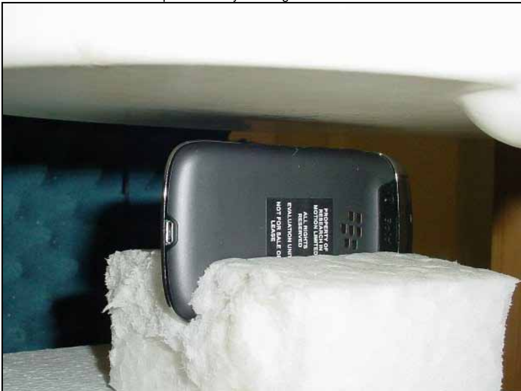
Photo 10: Test position body worn right side with 10 mm distance
