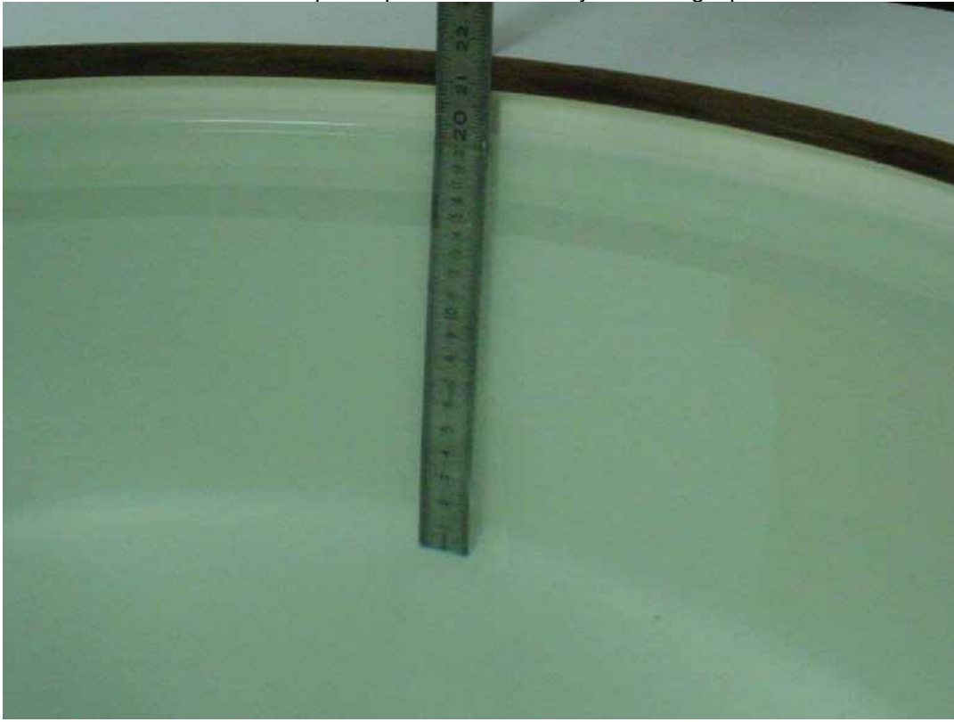
Photo 3: Liquid depth 2450 MHz body simulating liquid
