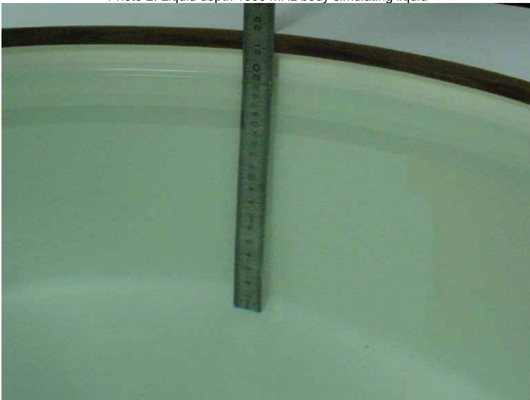
Photo 2: Liquid depth 1900 MHz body simulating liquid
