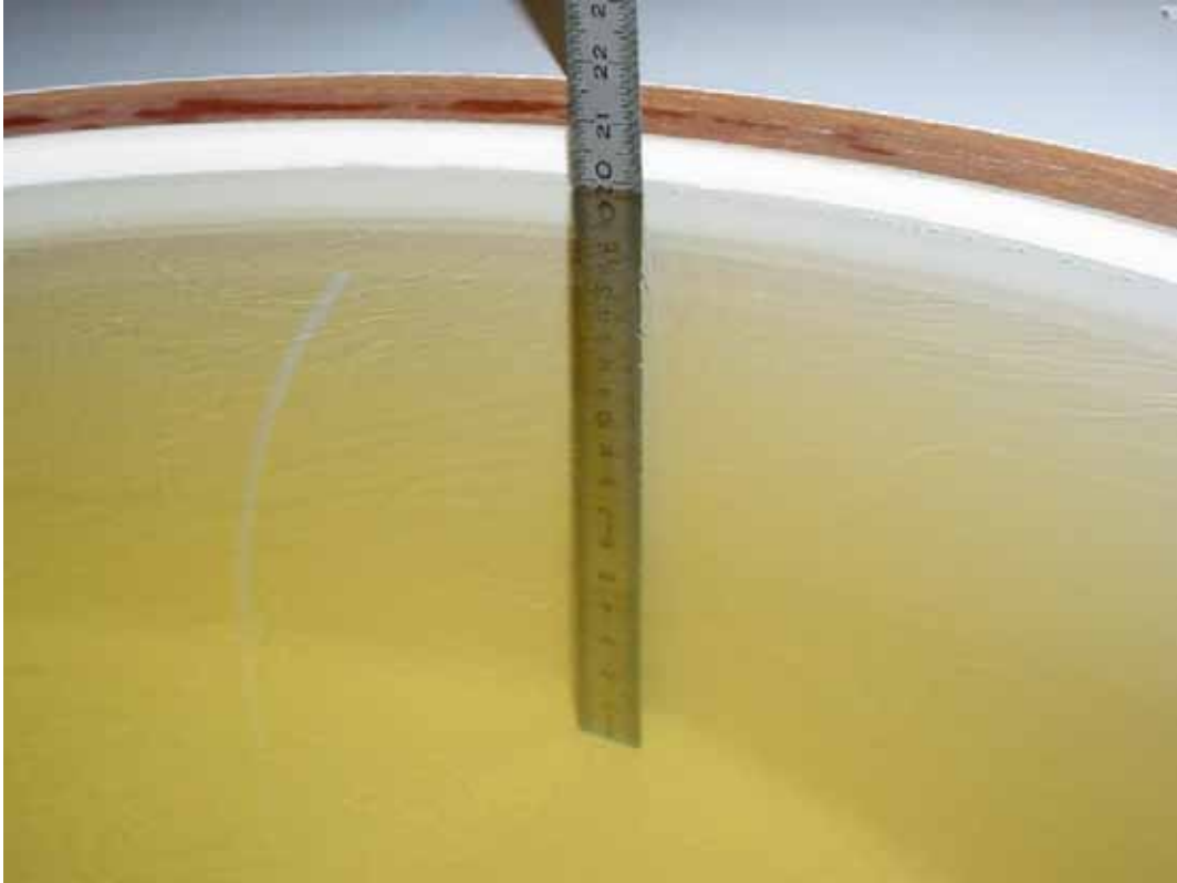
Photo 2: Liquid depth 1900 MHz body simulating liquid
