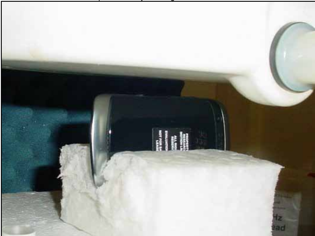
Photo 12: Test position body worn top side with 10 mm distance
