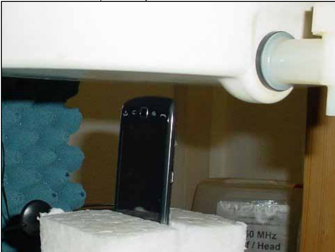
Photo 13: Test position body worn bottom side with 10 mm distance
