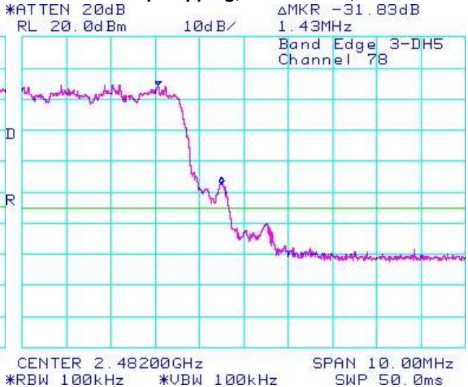
Figure 3-35: Band Edge Compliance
