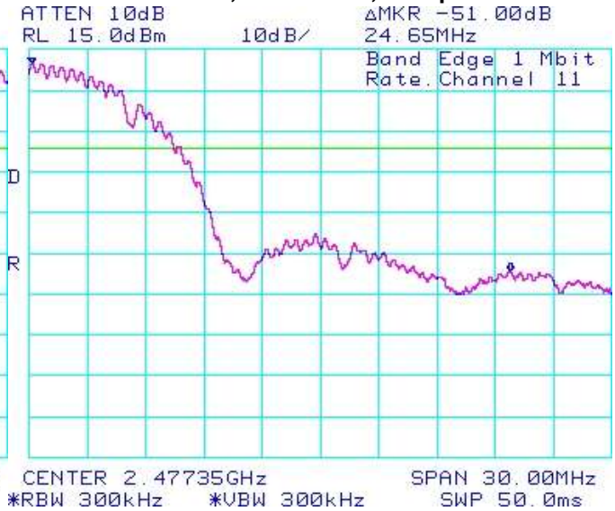
Figure 4-11: Band Edge Compliance
