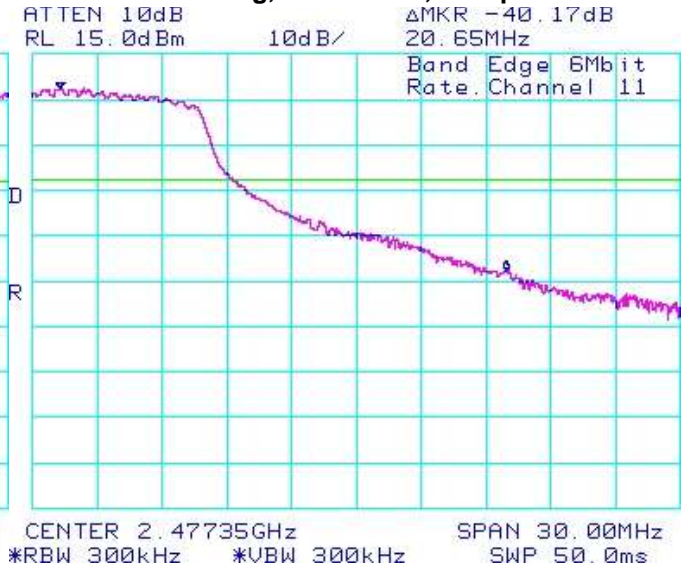
Figure 4-13: Band Edge Compliance
