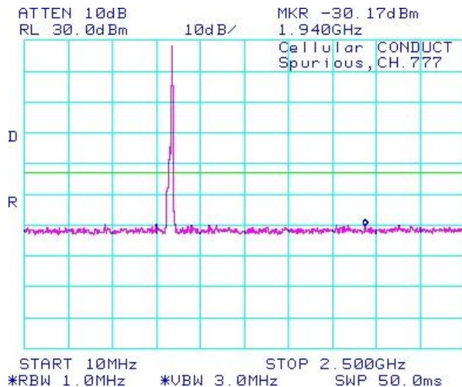
Figure 7-5b: Cellular, Spurious Conducted Emissions, High Channel
