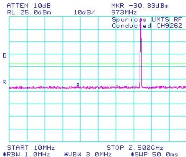
Figure 1-7c: BAND 2 Spurious Conducted Emissions, Low Channel
