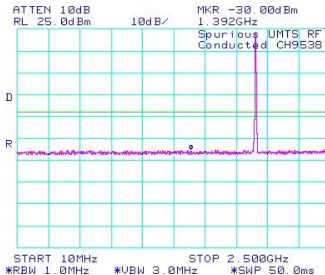
Figure 1-11c: BAND 2, Spurious Conducted Emissions, High Channel
