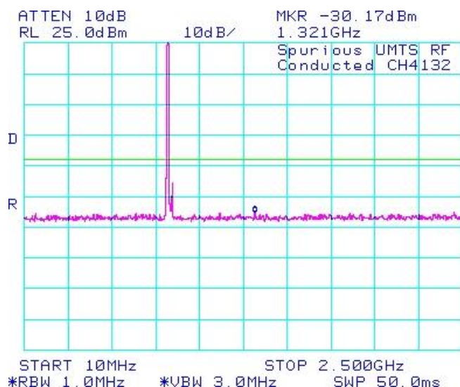
Figure 1-1c: Band 5, Spurious Conducted Emissions, Low channel
