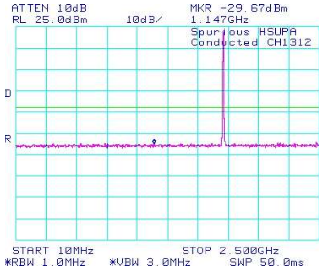
Figure 1-12c: Band 4 , Spurious Conducted Emissions, Low channel
