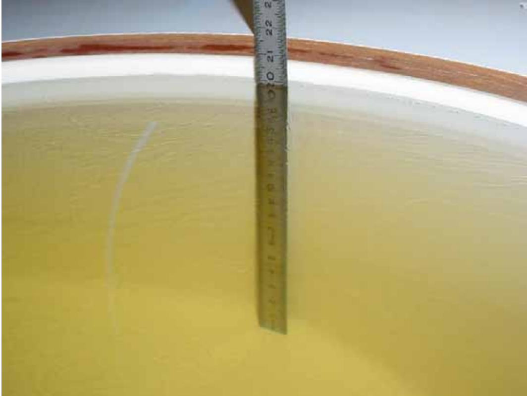
Photo 2: Liquid depth 1900 MHz body simulating liquid
