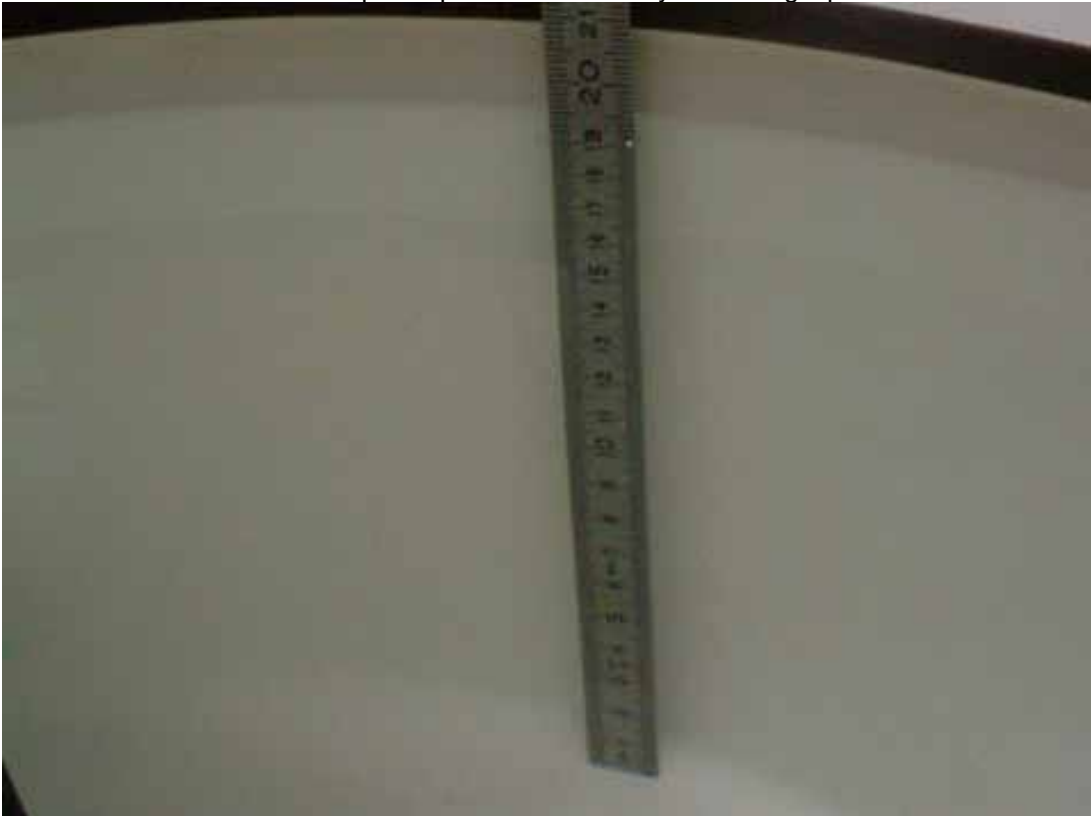
Photo 4: Liquid depth 2450 MHz body simulating liquid
