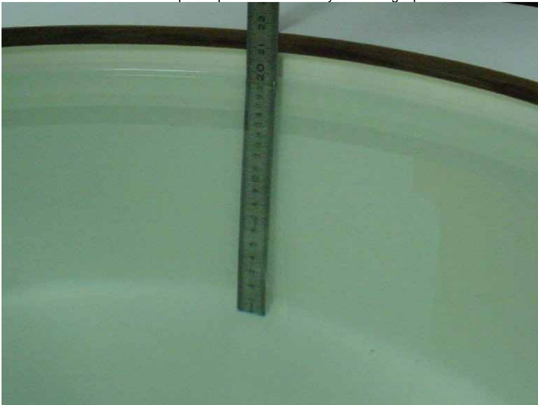
Photo 2: Liquid depth 1900 MHz body simulating liquid
