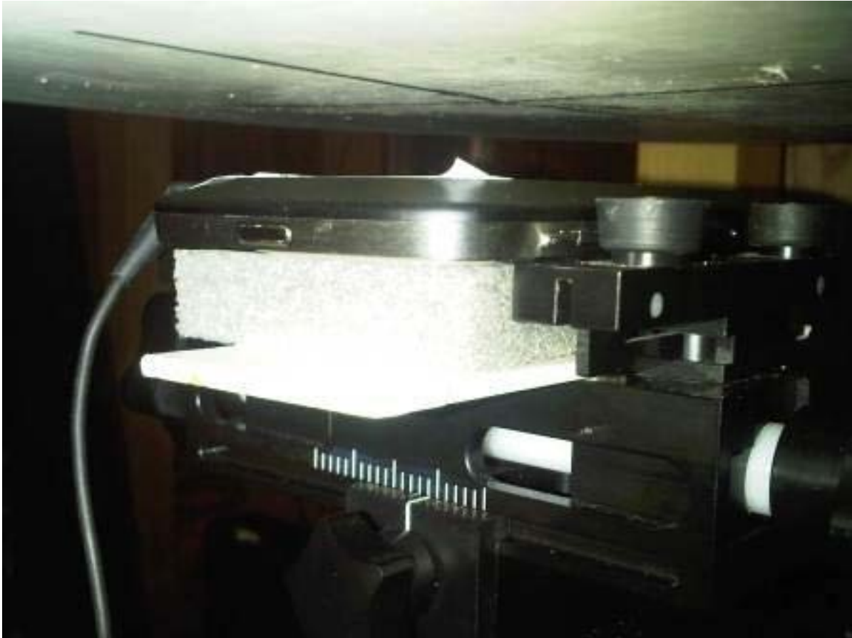
Figure E8. Body-worn configuration (No Holster, headset, back 15mm away)
