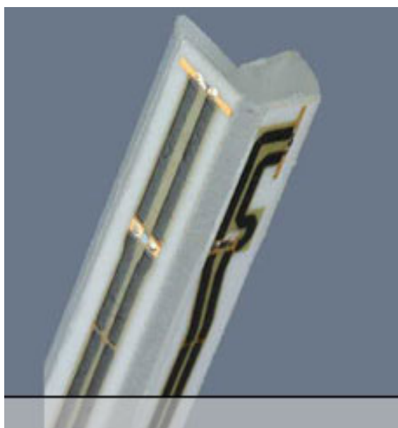
E-Field Probe (ER3DV6)
