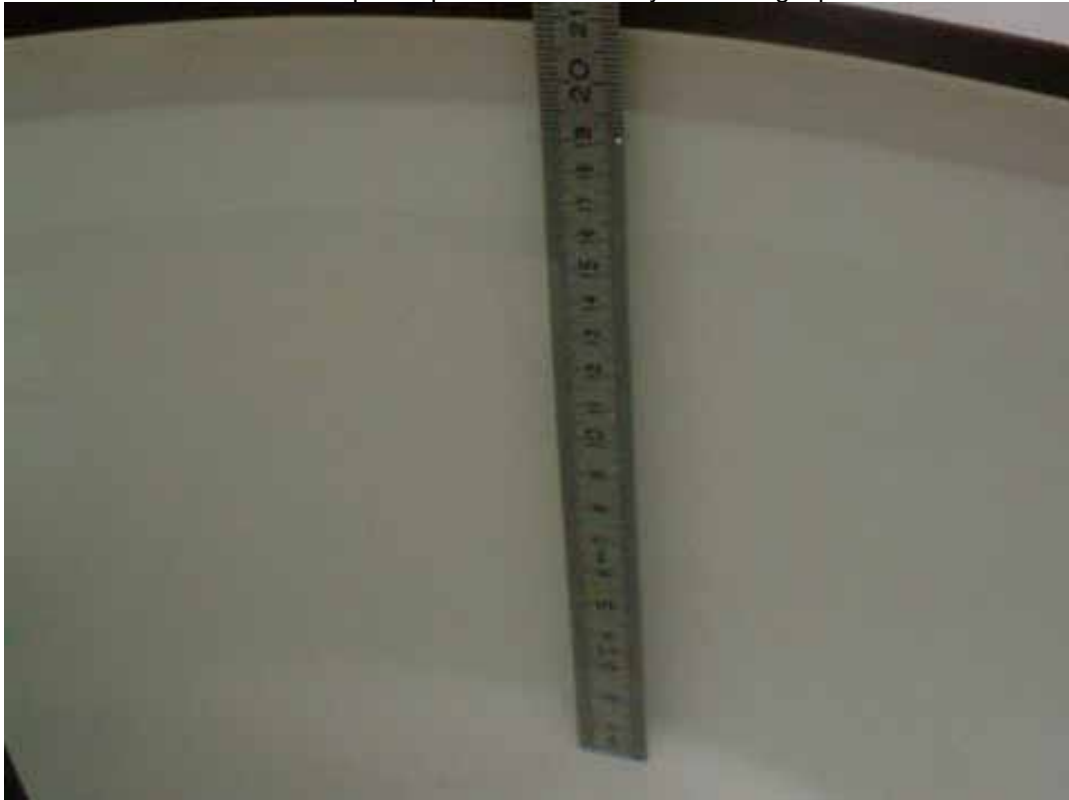
Photo 4: Liquid depth 2450 MHz body simulating liquid
