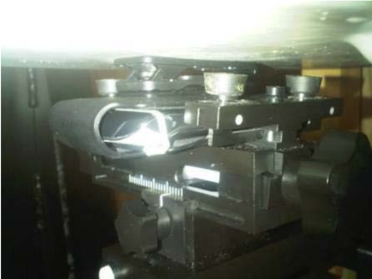
Figure E8. Body-worn configuration (Vertical Holster, front facing phantom)
