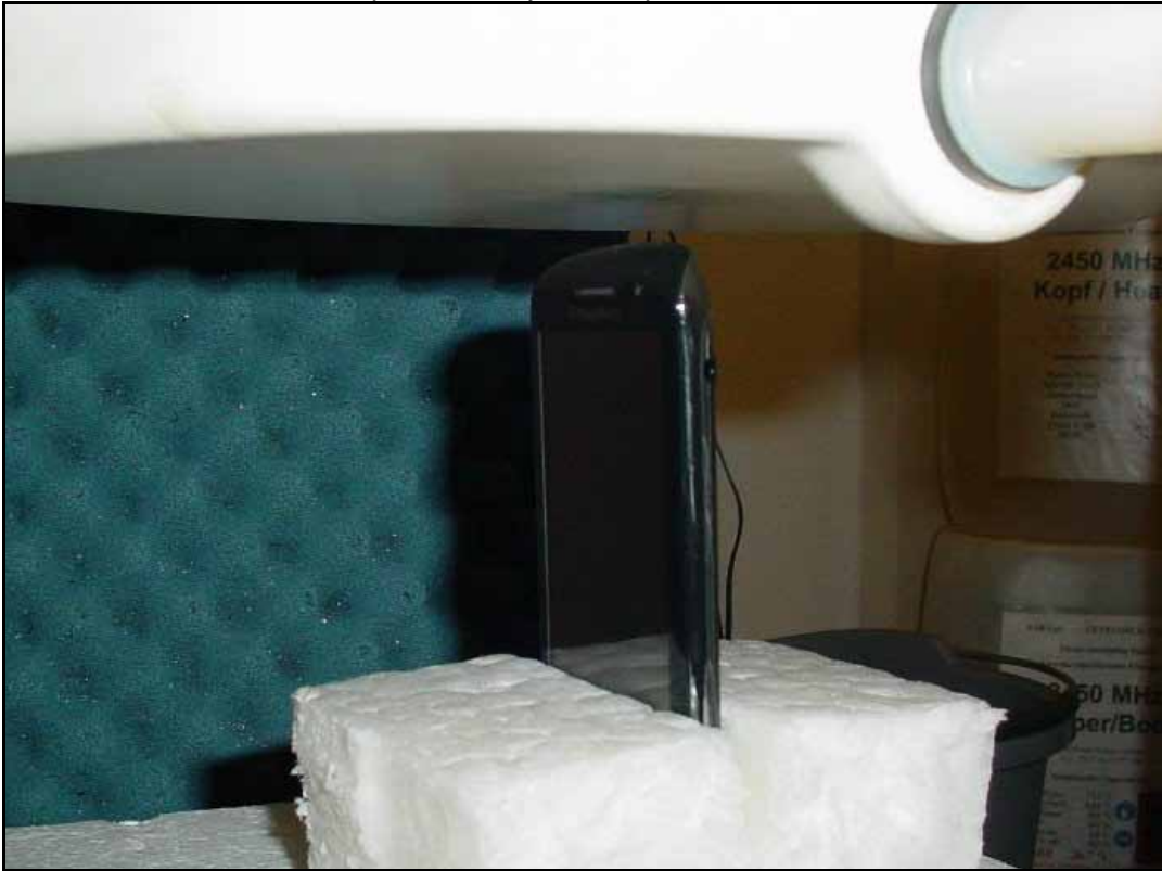
Photo 15: Test position body worn top side with 10 mm distance
