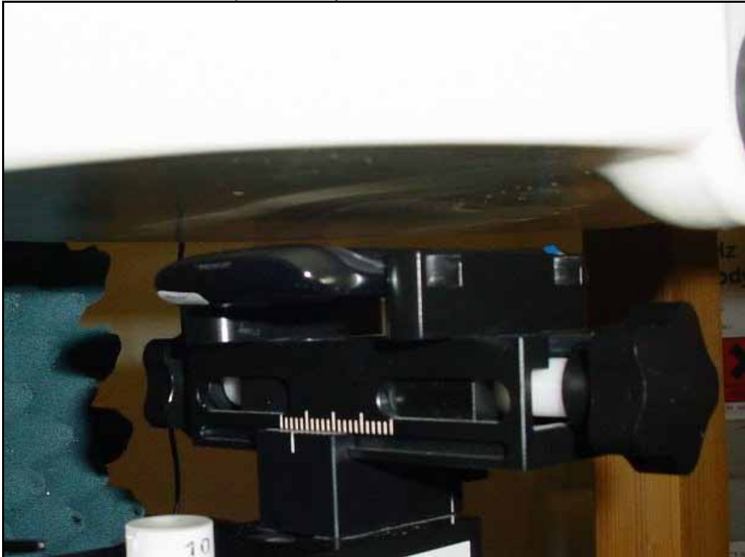
Photo 12: Test position body worn left side with 10 mm distance
