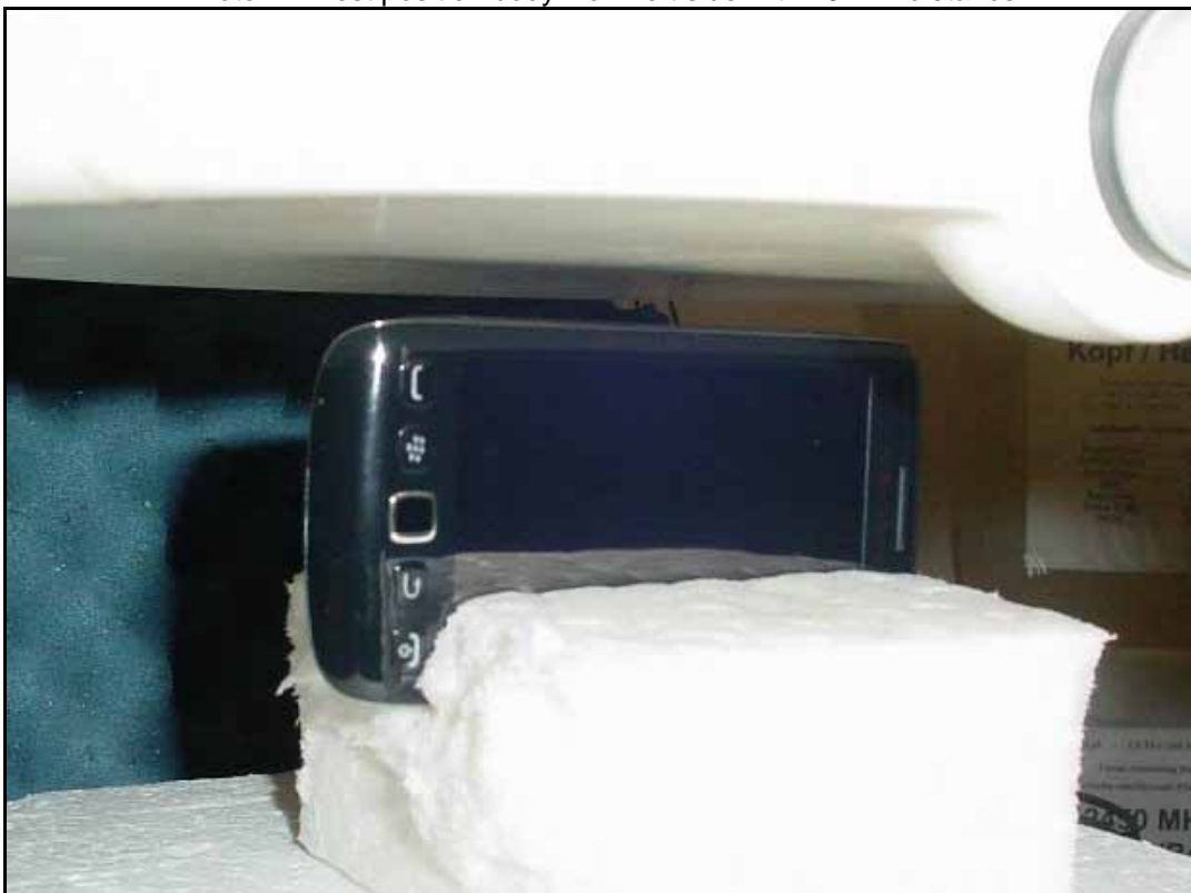
Photo 12: Test position body worn left side with 10 mm distance
