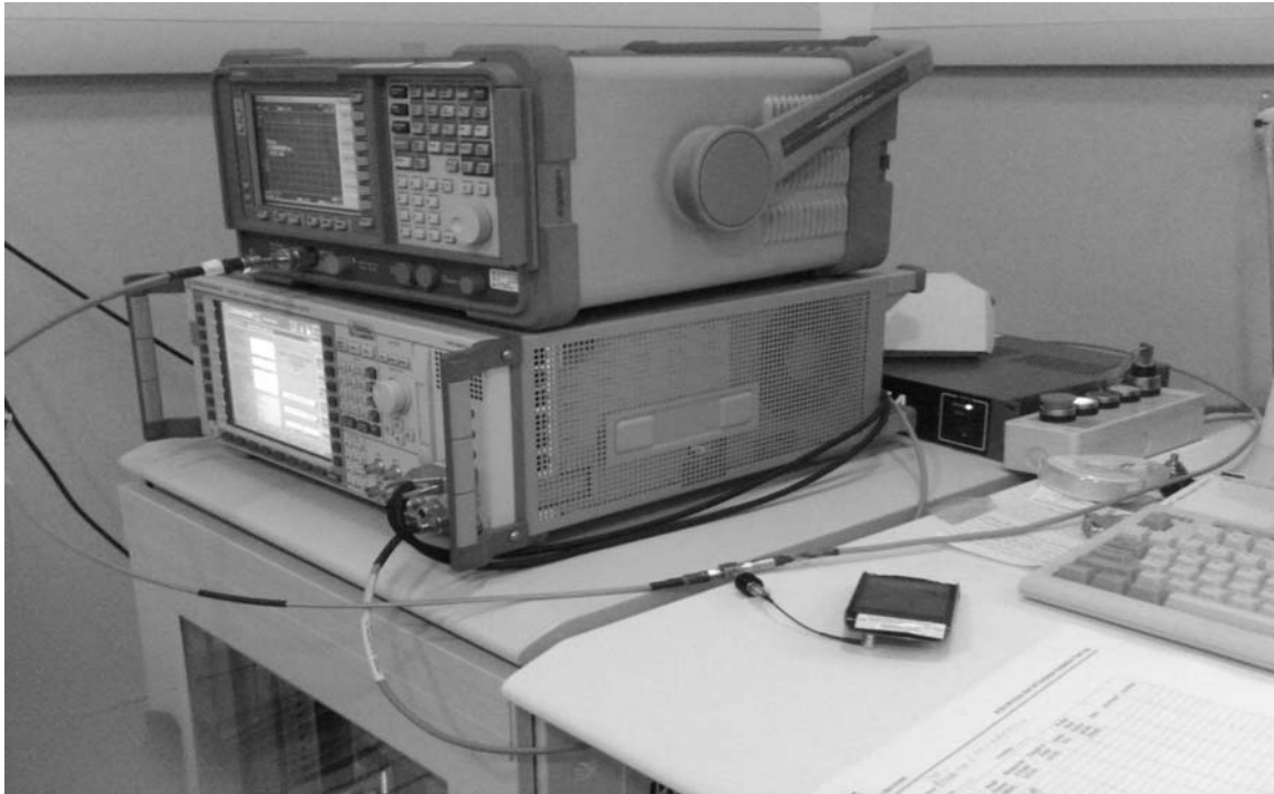
Figure 2 – Dipole Validation & Probe Modulation Factor measurement setup
