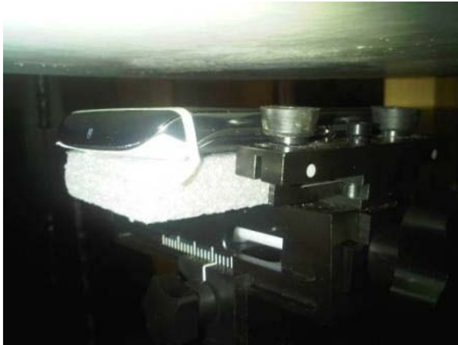
Figure E7. Body-worn configuration (No Holster, back side 25mm away from phantom)
