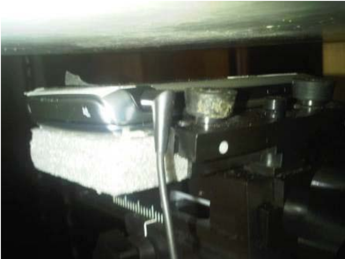
Figure E10. Body-worn configuration (No Holster, Headset #1, 15mm away, back facing phantom)
