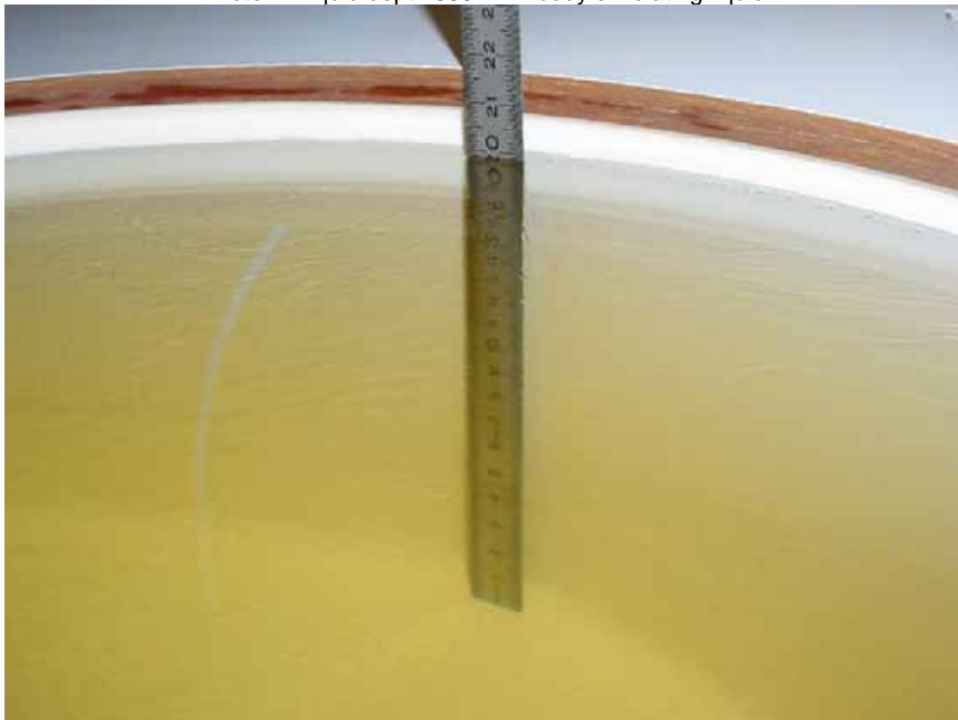
Photo 1: Liquid depth 850 MHz body simulating liquid
