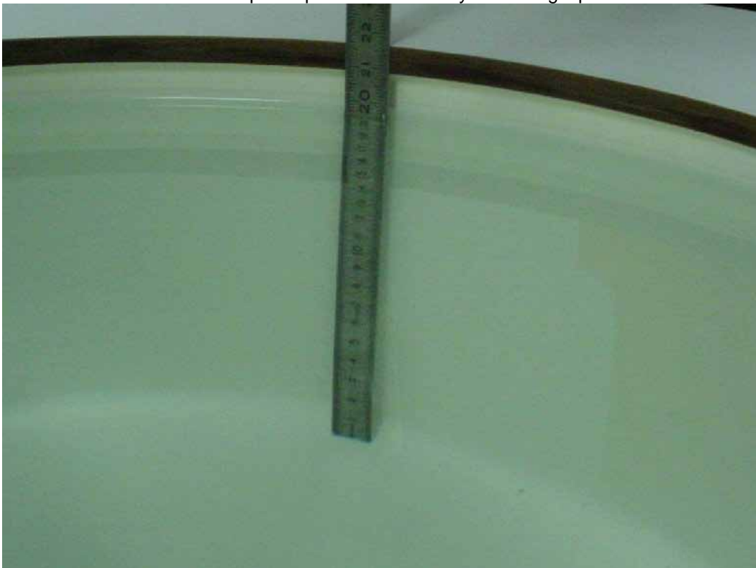
Photo 3: Liquid depth 2450 MHz body simulating liquid
