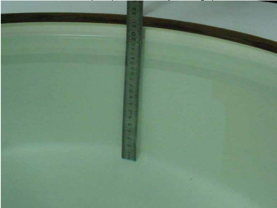
Photo 3: Liquid depth 2450 MHz body simulating liquid
