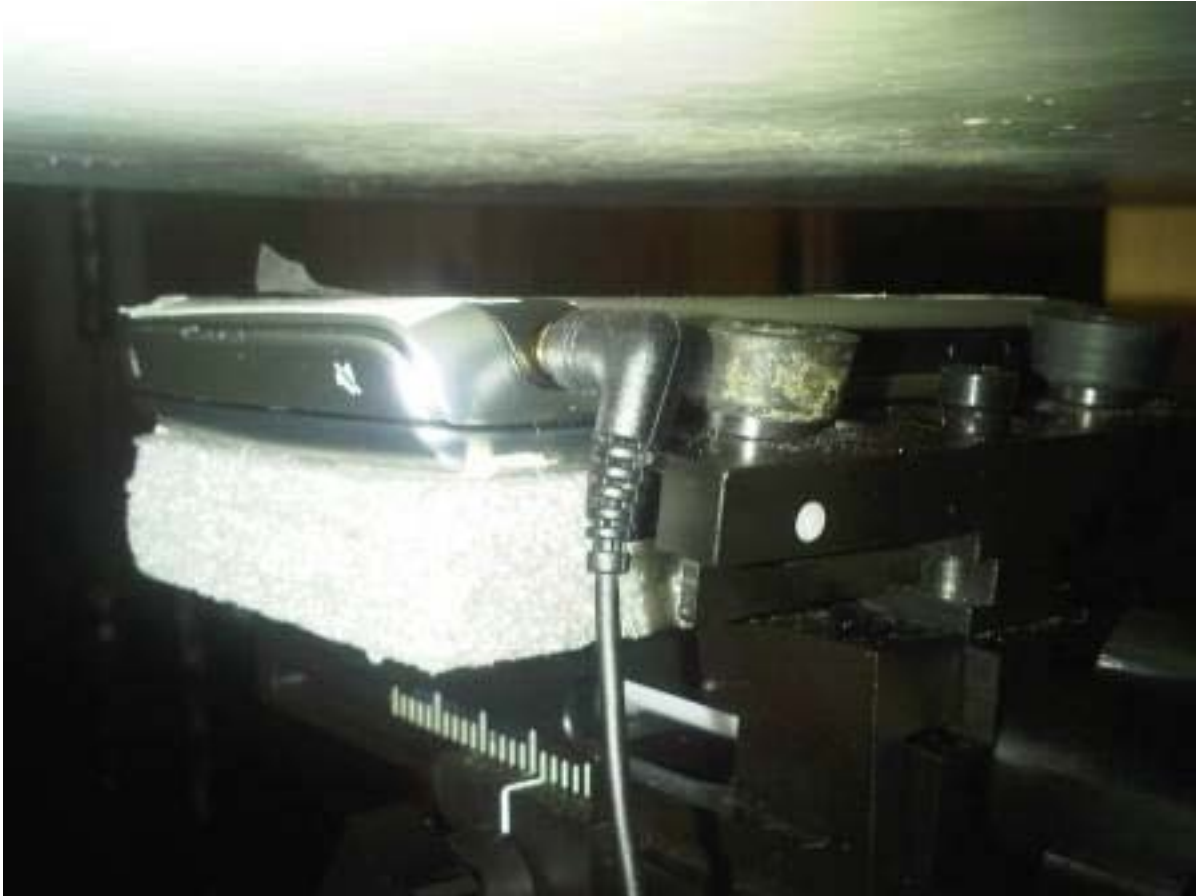
Figure E11. Body-worn configuration (No Holster, Headset #2, 15mm away, back facing phantom)
