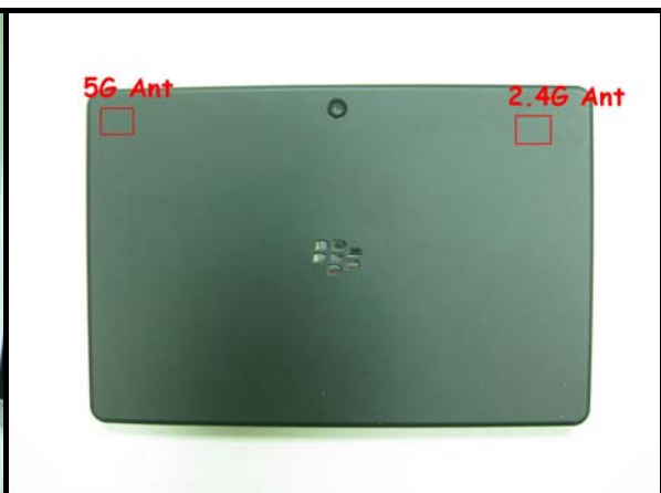
DESCRIPTION OF ANTENNA LOCATION
