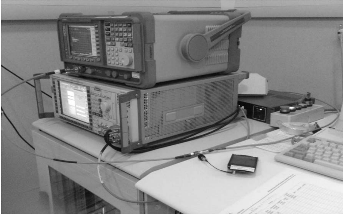
Figure 2 – Dipole Validation & Probe Modulation Factor measurement setup
