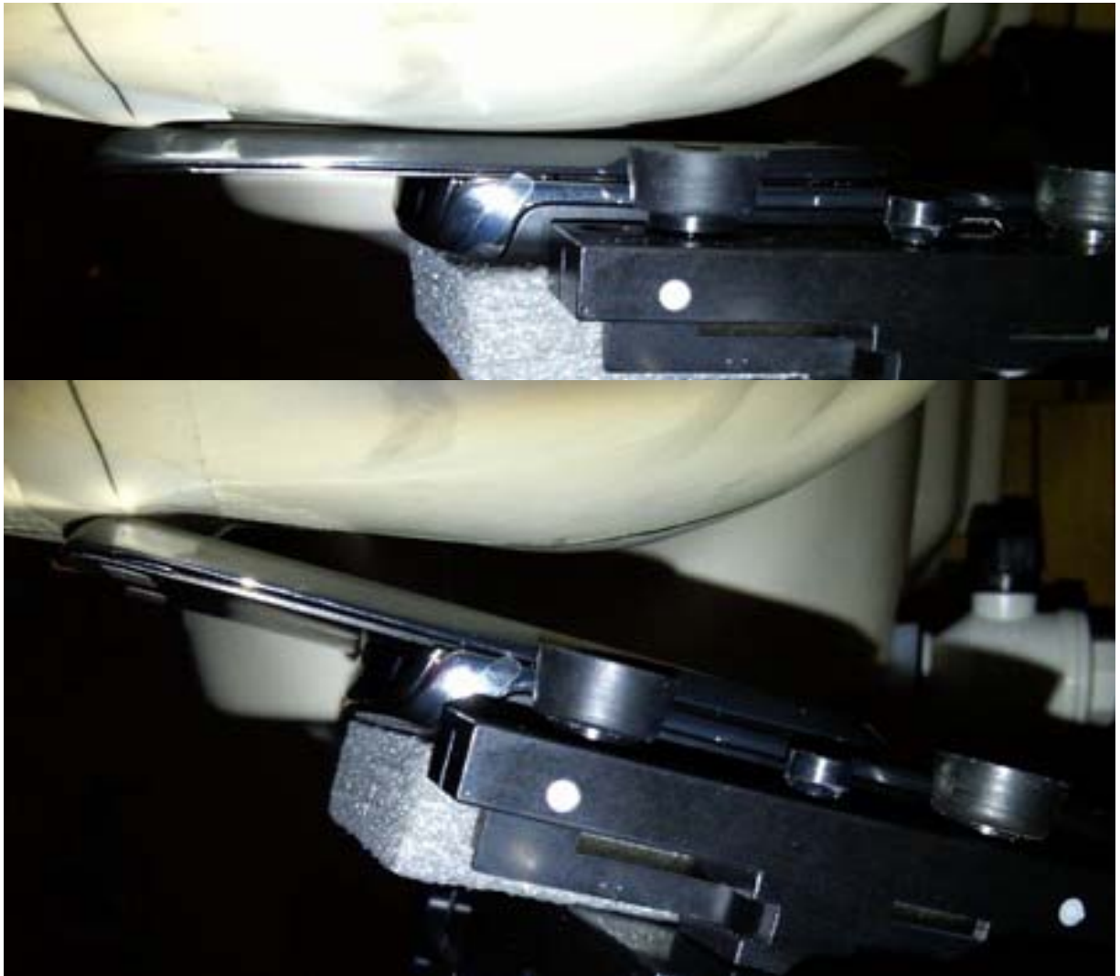
Figure E5. Head configuration (Right Touch/Tilt/Slider Open)
