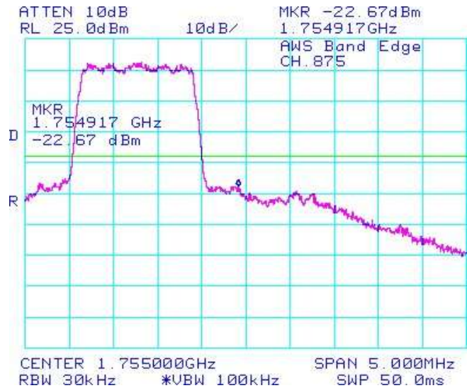
Figure 1-20c: CDMA AWS Band Edge High Channel
