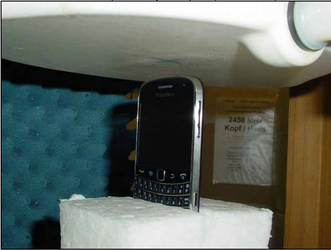
Photo 15: Test position body worn top side (10 mm distance)
