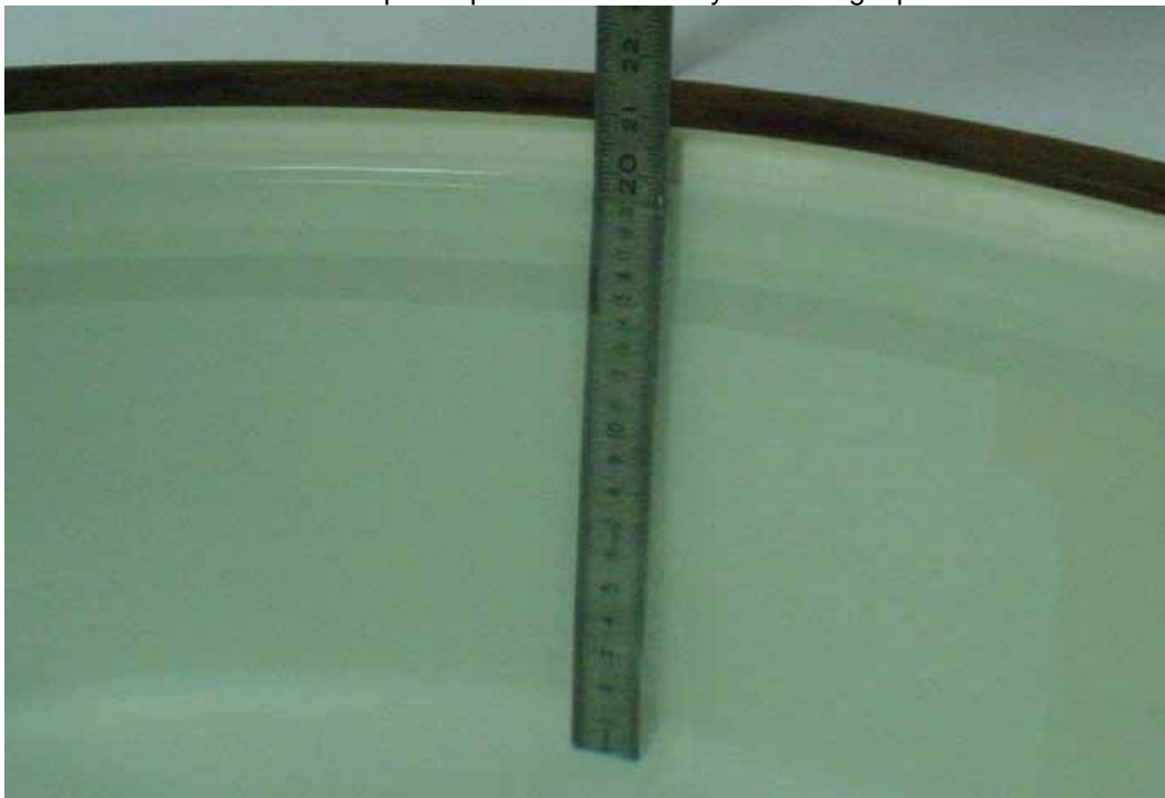
Photo 3: Liquid depth 2450 MHz body simulating liquid
