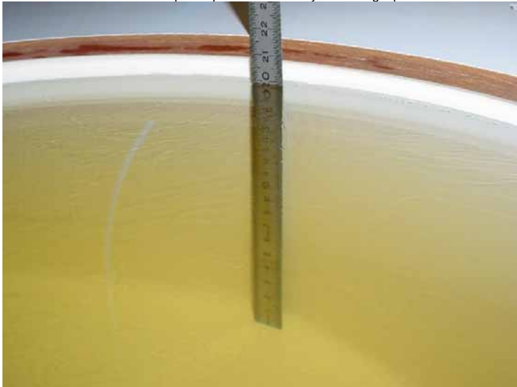
Photo 1: Liquid depth 850 MHz body simulating liquid
