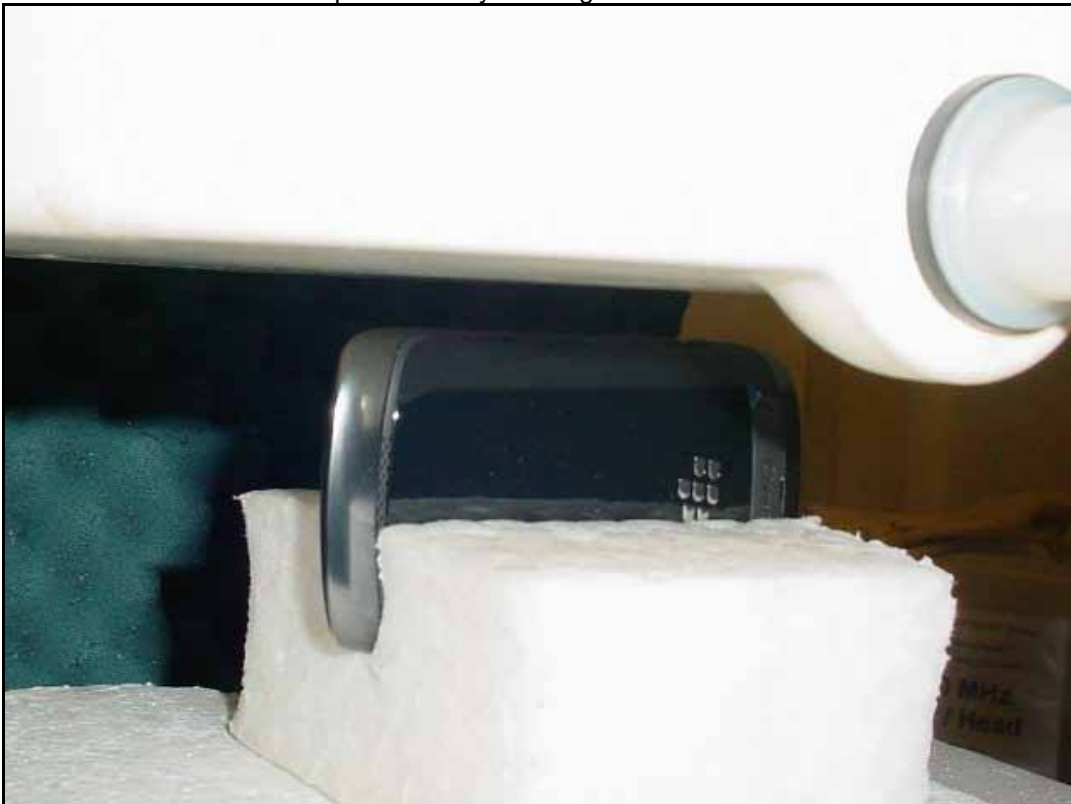
Photo 12: Test position body worn right side with 10 mm distance
