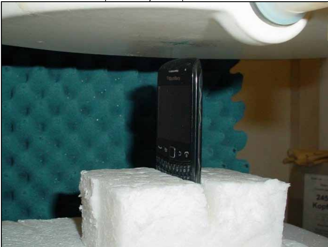
Photo 14: Test position body worn top side with 10 mm distance
