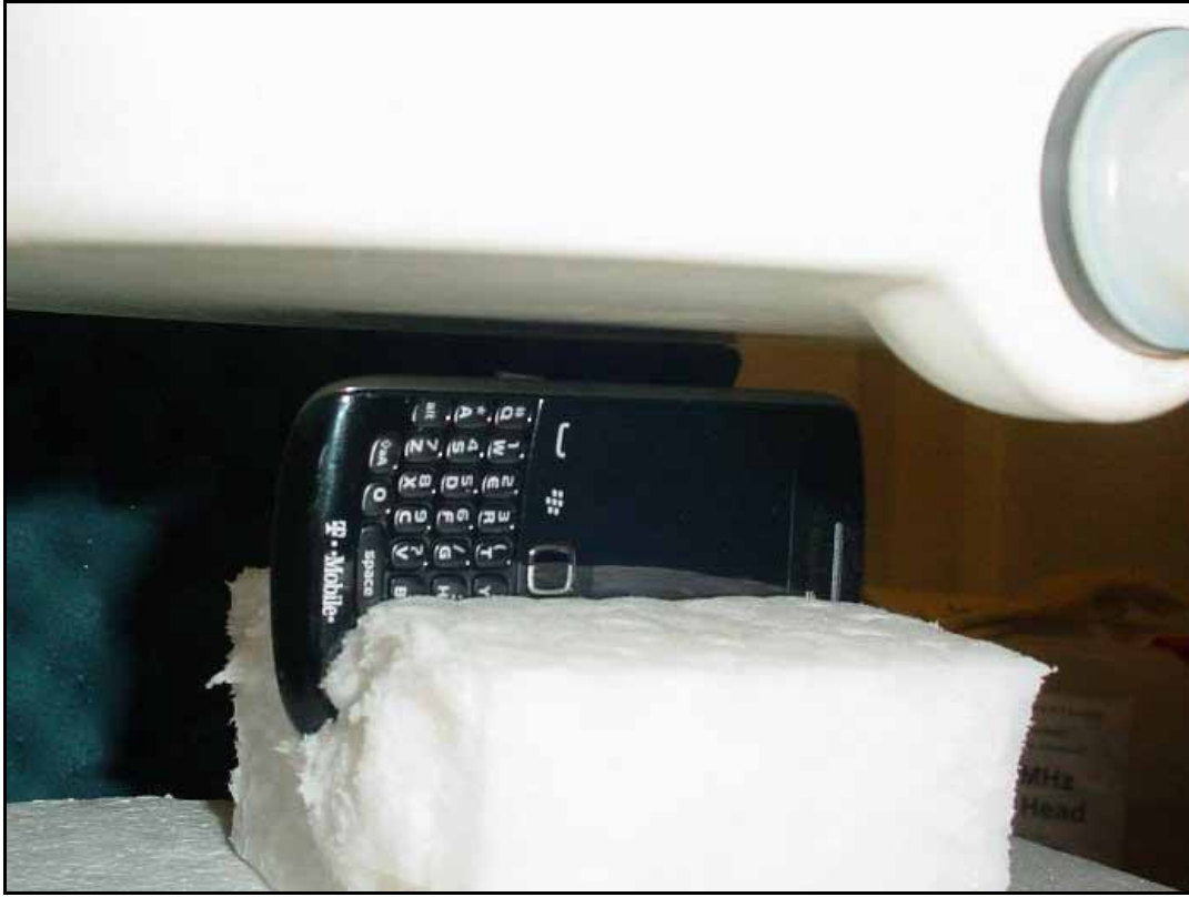
Photo 12: Test position body worn right side with 10 mm distance
