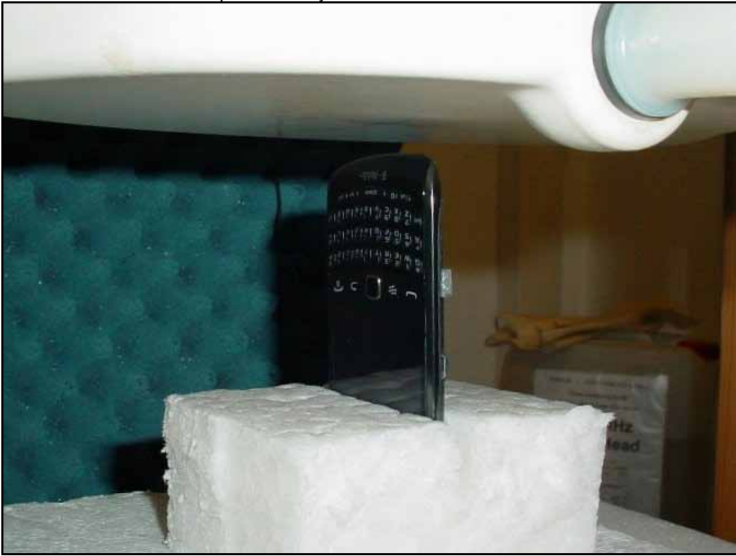
Photo 14: Test position body worn top side with 10 mm distance
