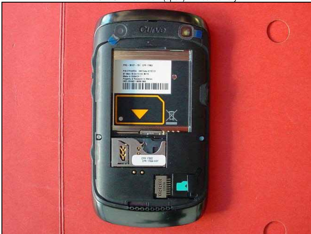
Photo 6: DUT - rear view (open) without battery
