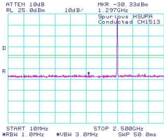
Figure 1-16c: Band 4 , Spurious Conducted Emissions, High Channel
