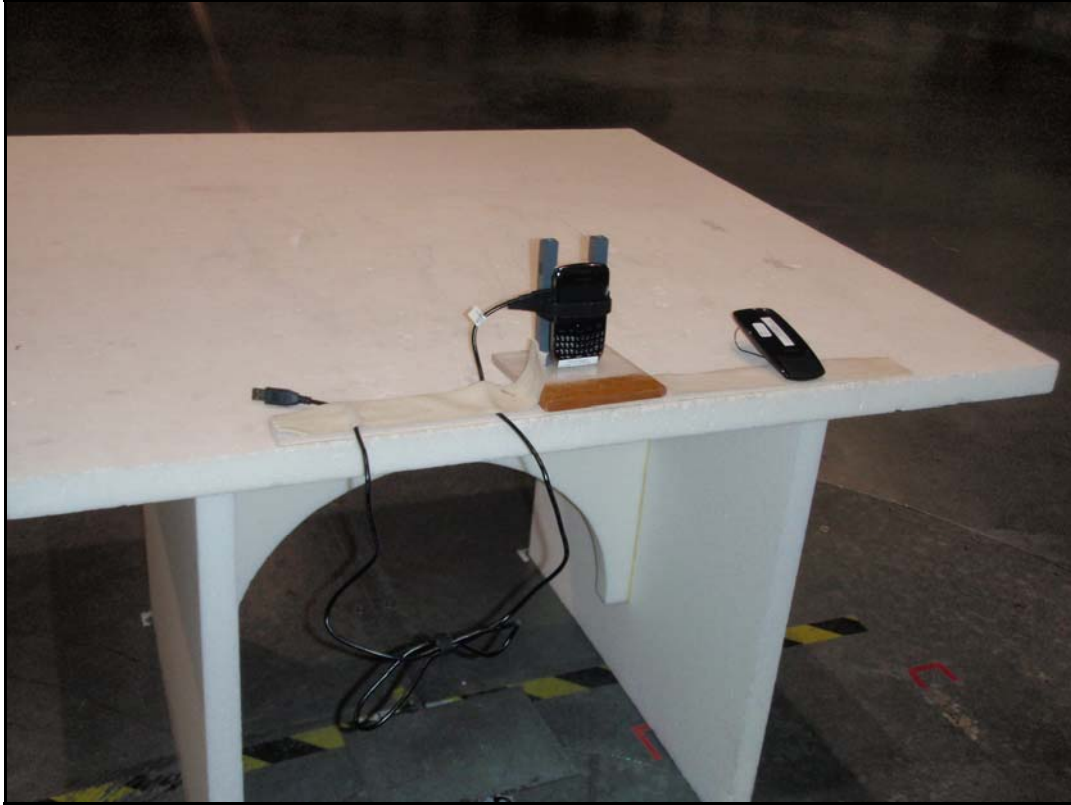
Photo 2: radiated emission < 1 GHz (Set 1 / Op 1)
