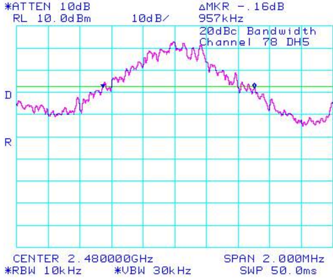
Figure 3-3: 20 dB Bandwidth Single freq., Static PBRs, DH5
