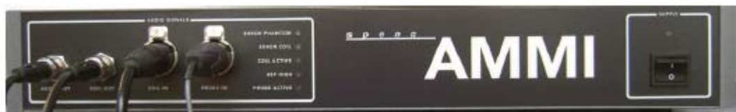
Figure 5.2. The Audio band Magnetic field Measuring Instrument (AMMI)
