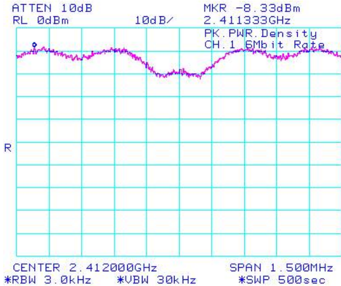
Figure 4-19: Peak Power Spectral Density 802.11g, Channel 1, 6 Mbps
