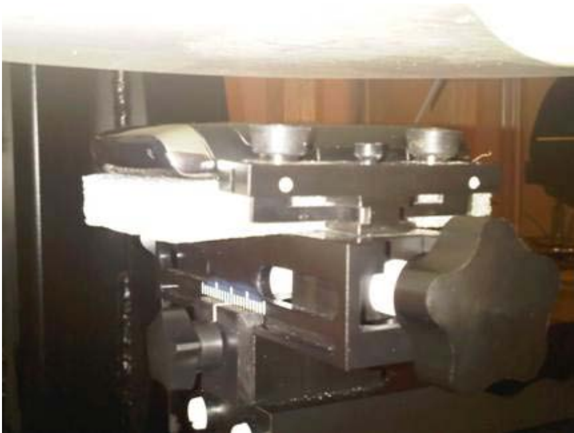
Figure E16. Body-worn configuration (No Holster, 25 mm away, back facing phantom)
