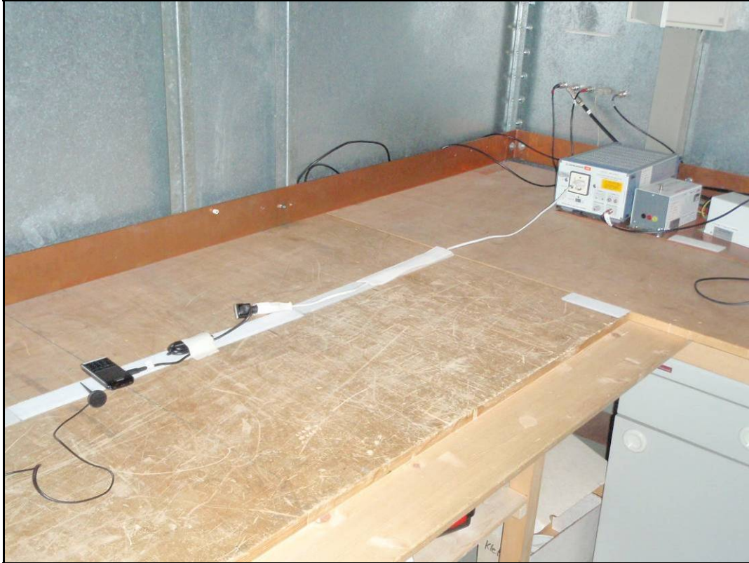
Photo 2: setup of radiated Emission < 1 GHz (set. 2)
