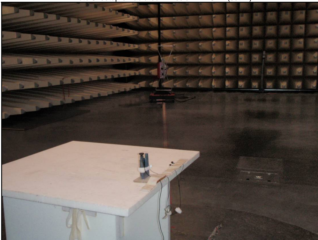
Photo 8: setup of radiated Emission < 1 GHz (set. 4)
