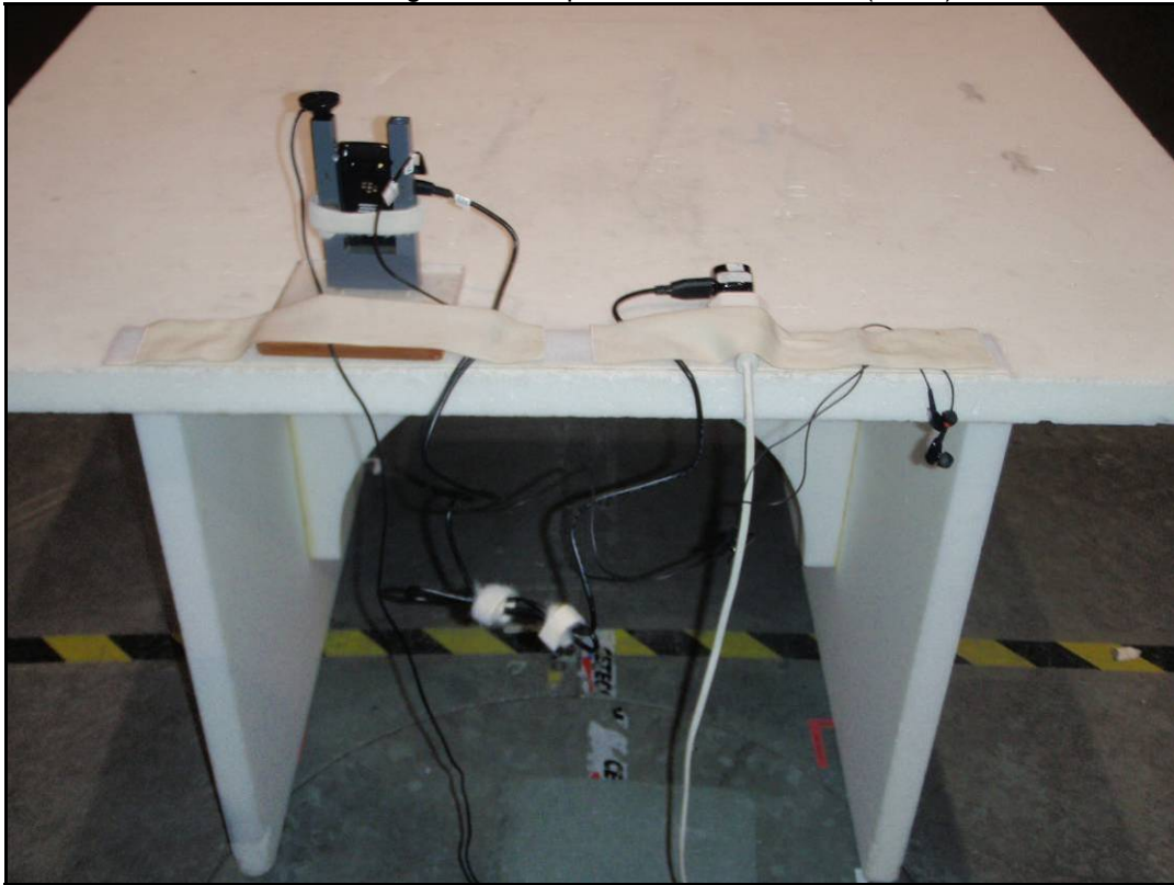
Photo 8: setup of radiated Emission < 1 GHz (set. 4)
