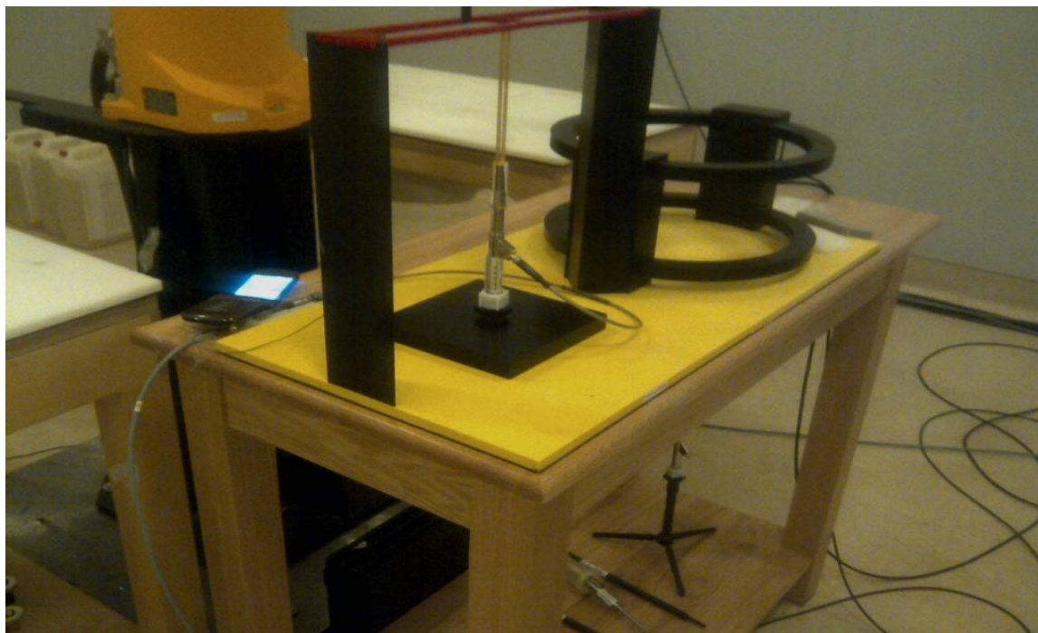
Figure 2 – Dipole Validation & Probe Modulation Factor measurement setup
