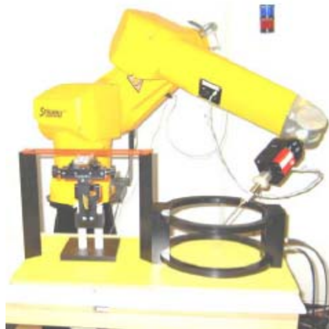
Figure 5.1: T-Coil set up with HAC Test Arch with Helmholtz Coil (AMCC)
