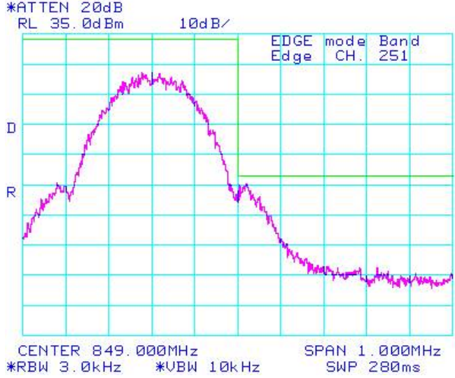
Figure 1-36a: GSM850 band High Channel Mask in EDGE mode
