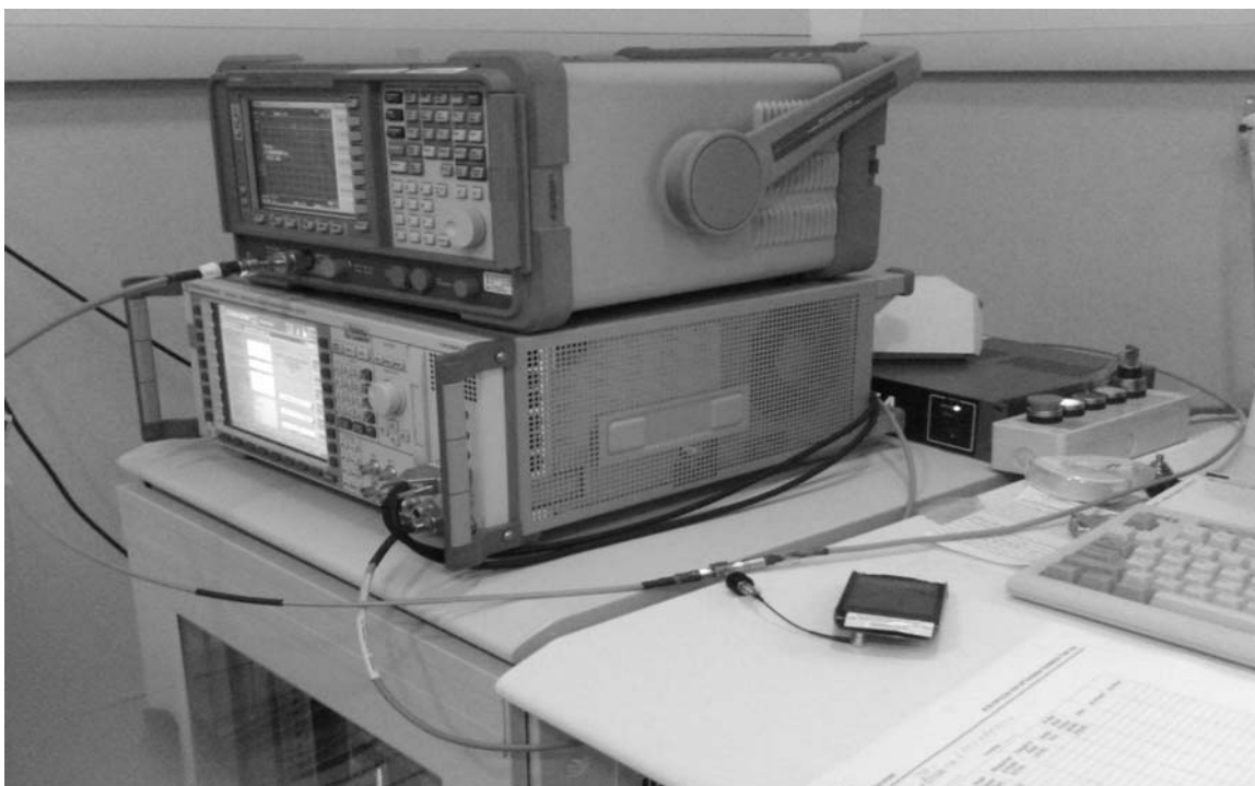
Figure 2 – Dipole Validation & Probe Modulation Factor measurement setup
