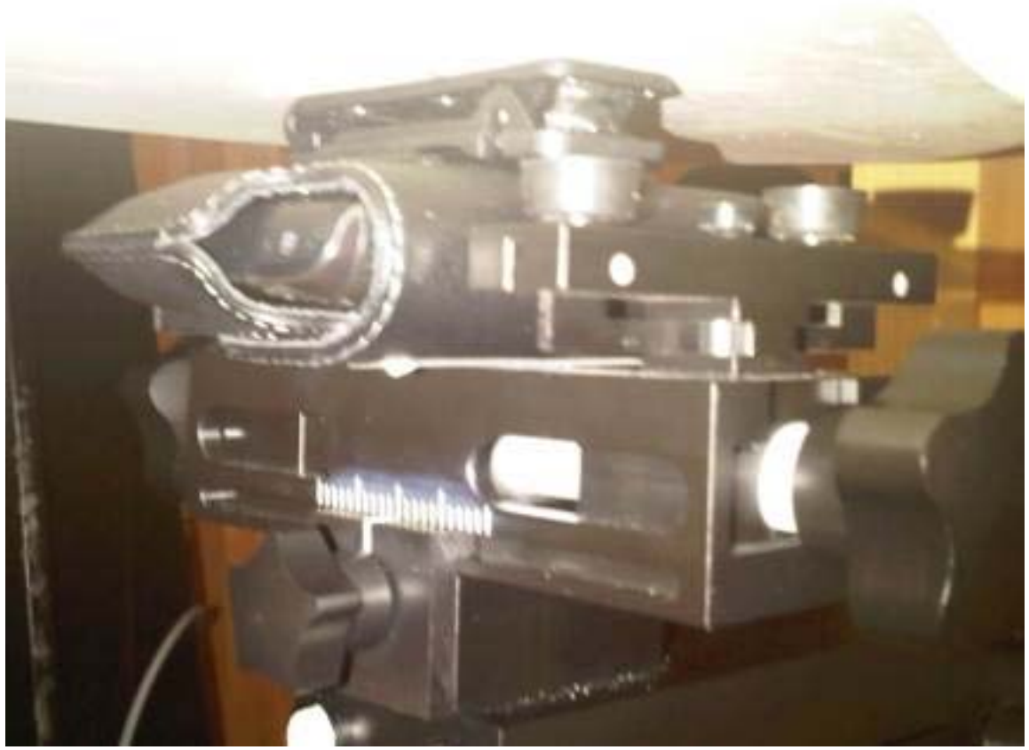
Figure E11. Body-worn configuration (Horizontal Holster, front facing phantom)
